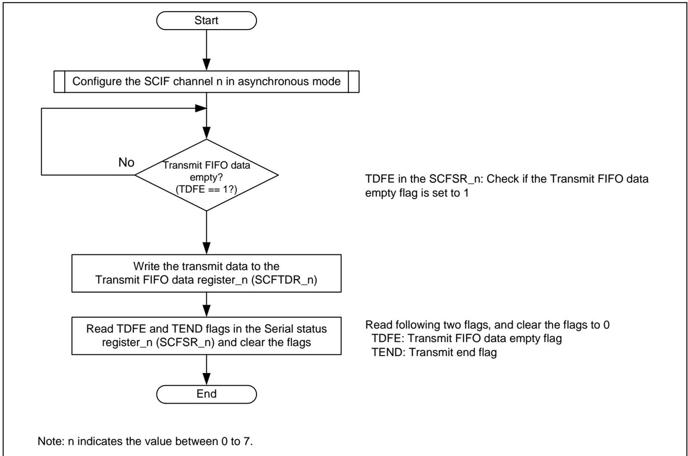
Figure 4 Flow Chart of the Transmission in Asynchronous Mode
