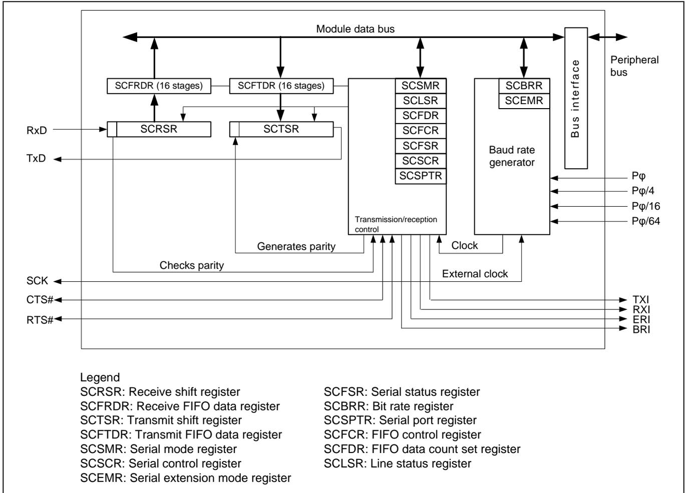
Figure 1 SCIF Block Diagram
