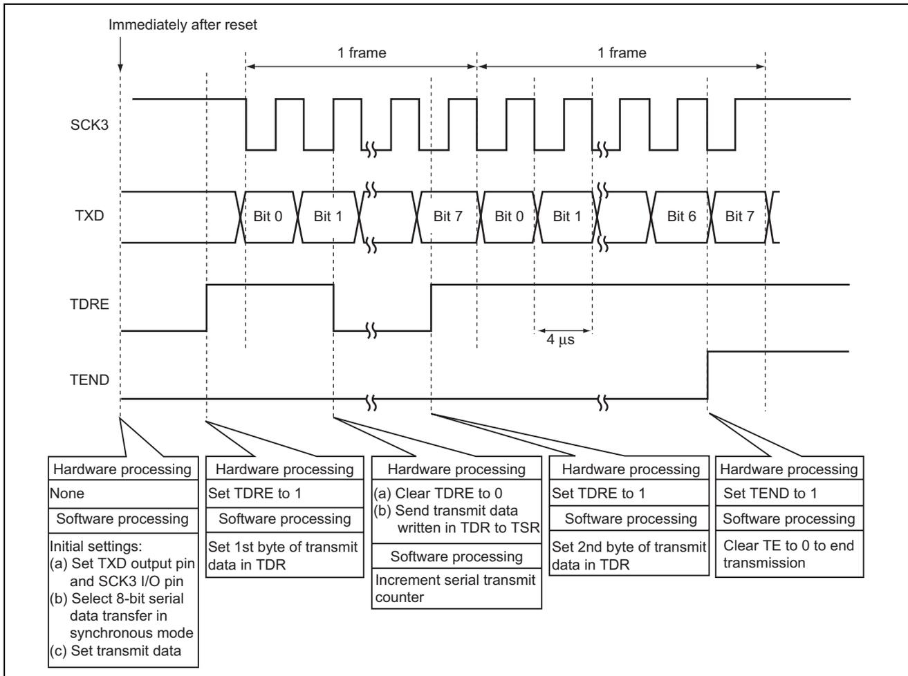
Figure 3 Operation Principle: Serial Data Transmission in Synchronous Mode
