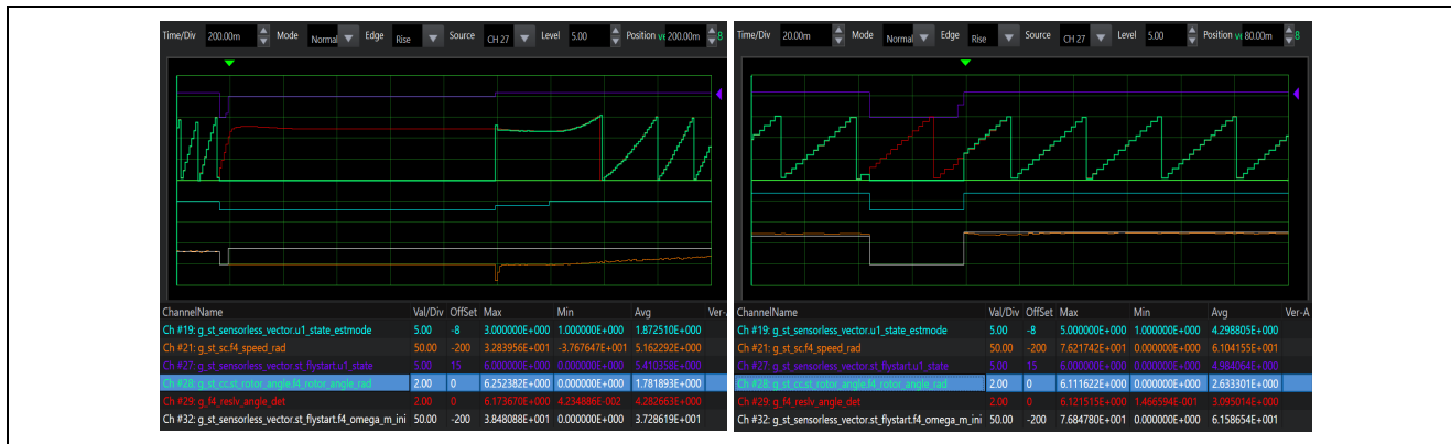
Figure 12-9 Current Waveforms during Operation in Flying Start Mode (Left: Active Braking; Right: Flying Start)
