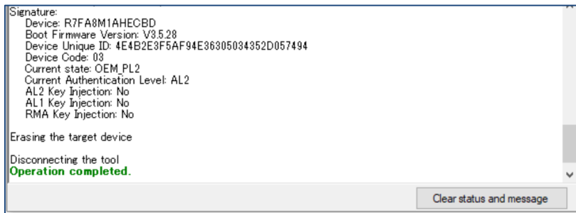
Figure 93. MCU is Successfully Initialized
