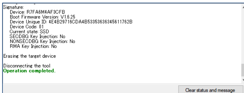
Figure 87. MCU is Successfully Initialized
