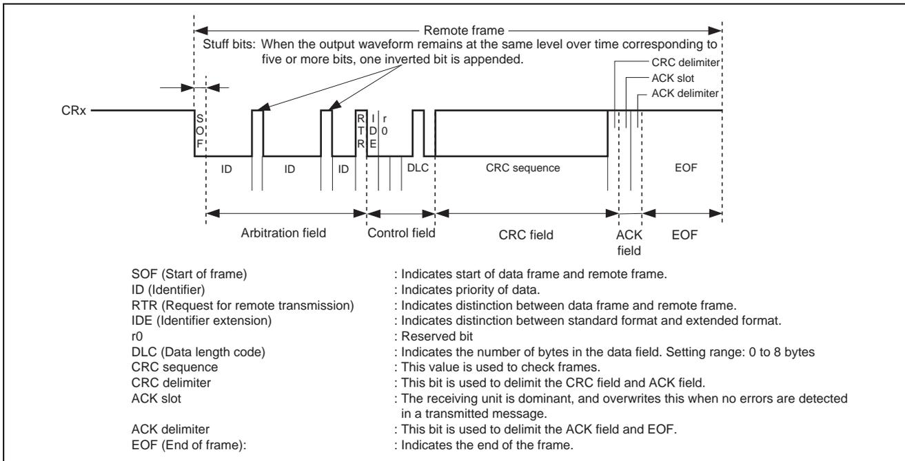
**Figure 5 Waveform for Remote Frame Reception by the RCAN-TL1**
