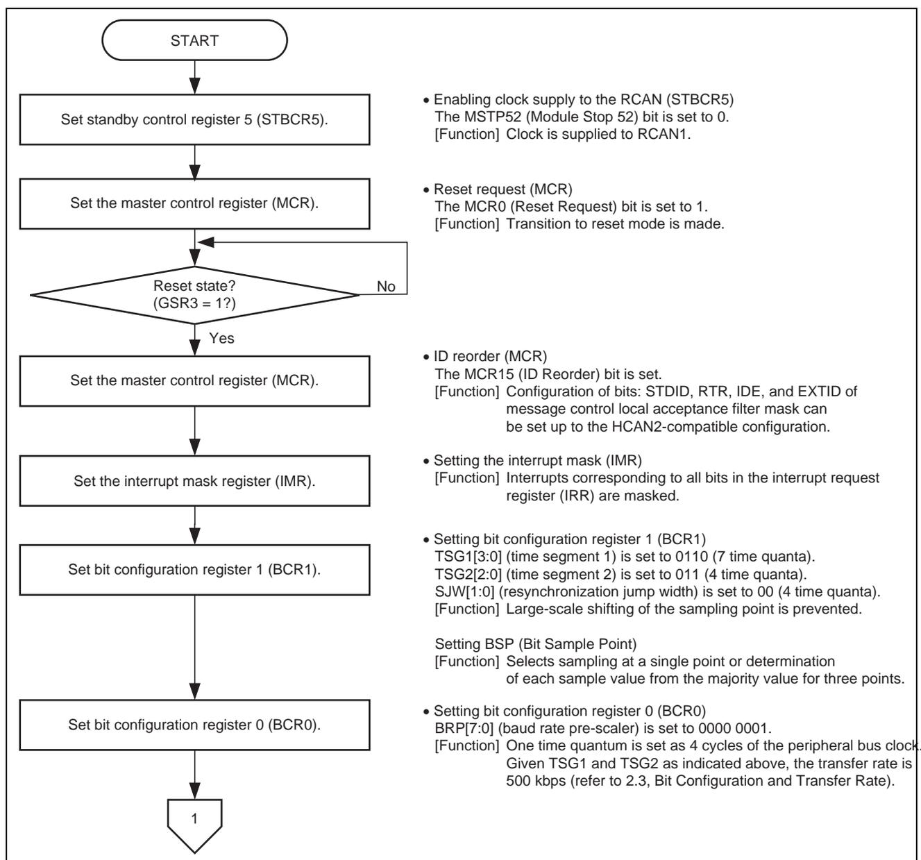
Figure 2 Example of Initialization Flow for the RCAN-TL1 Module (1)
