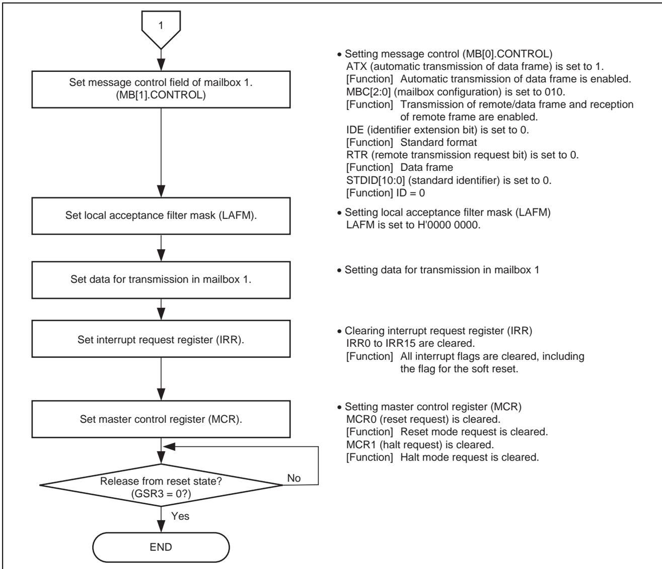
Figure 3 Example of Initialization Flow for the RCAN-TL1 Module (2)
