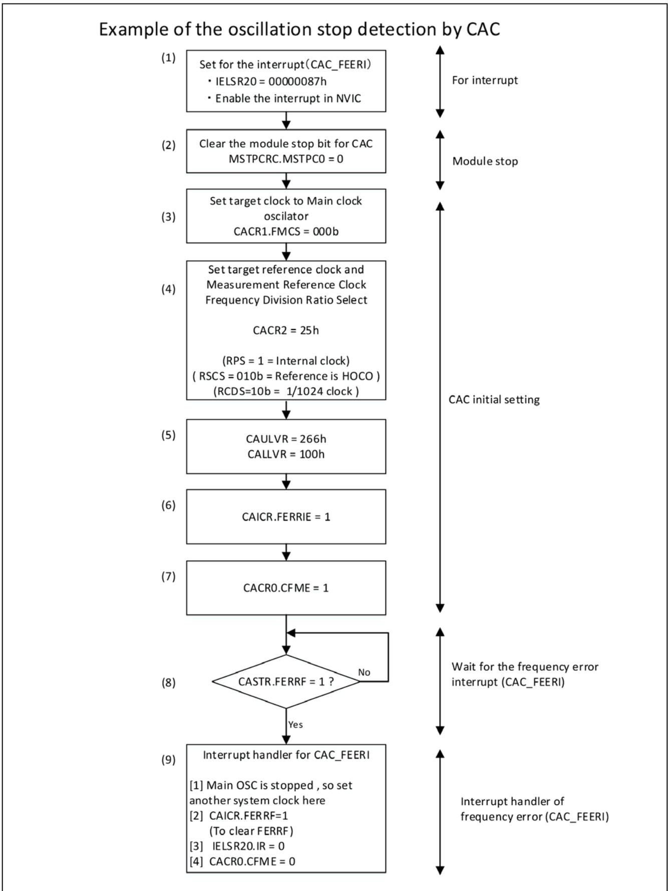
**Figure 4 CAC Frequency Error Interrupt for Oscillation Stop Detection (Reference Clock is 16 MHz HOCO)**
