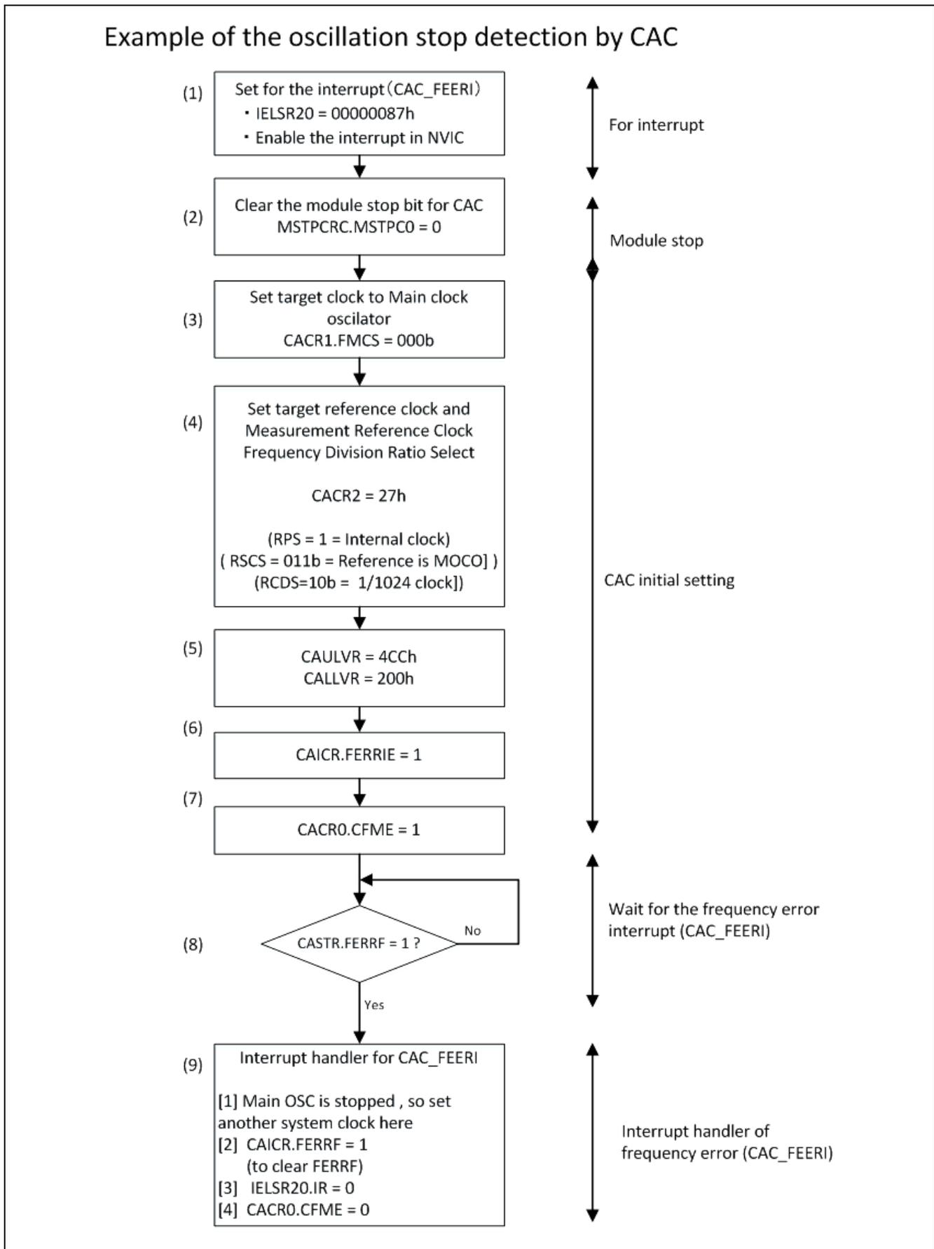
**Figure 3 CAC frequency error interrupt for oscillation stop detection (Reference Clock is 8 MHz MOCO)**
