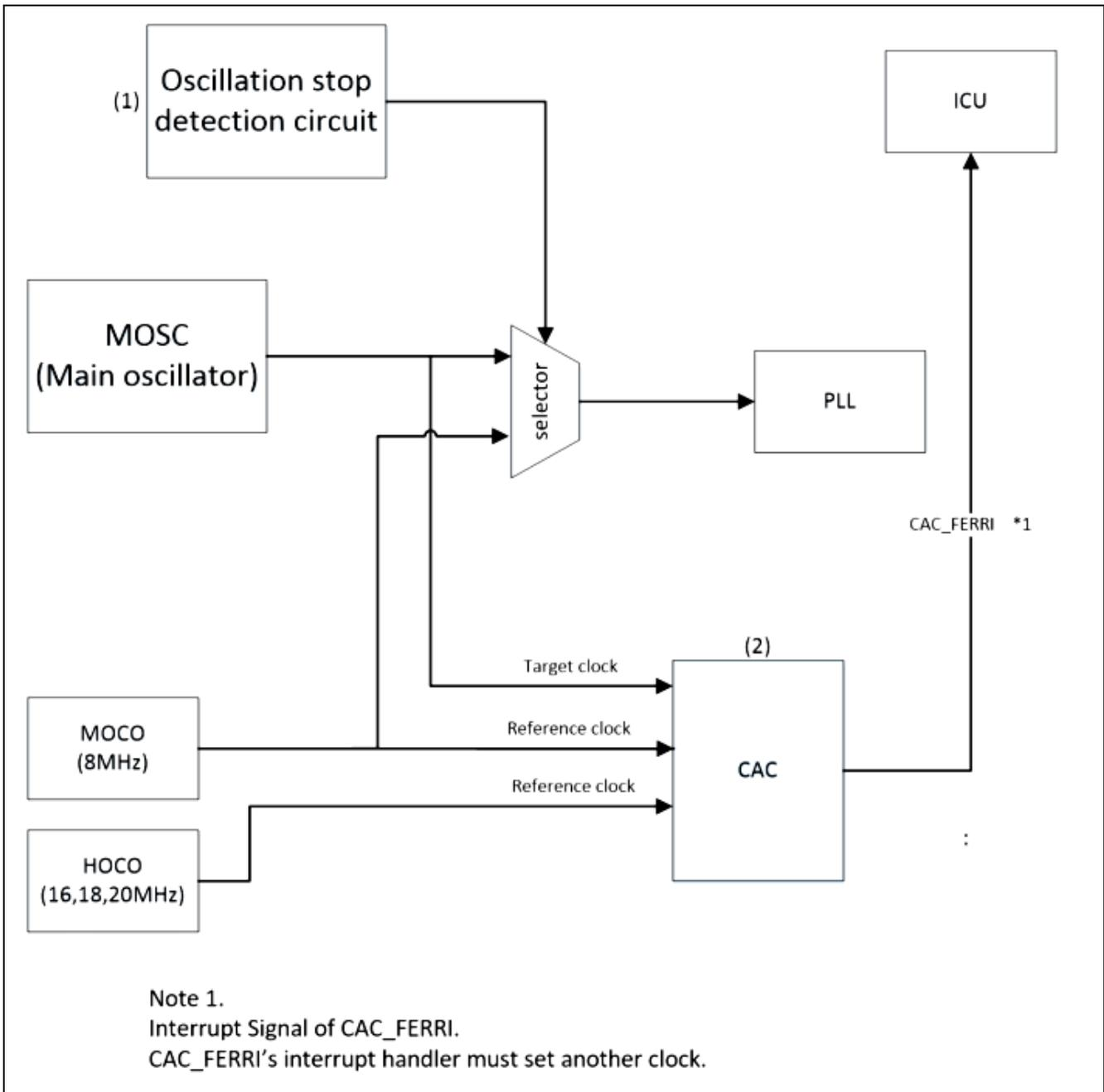
Figure 1 Oscillation stop detection by CAC
