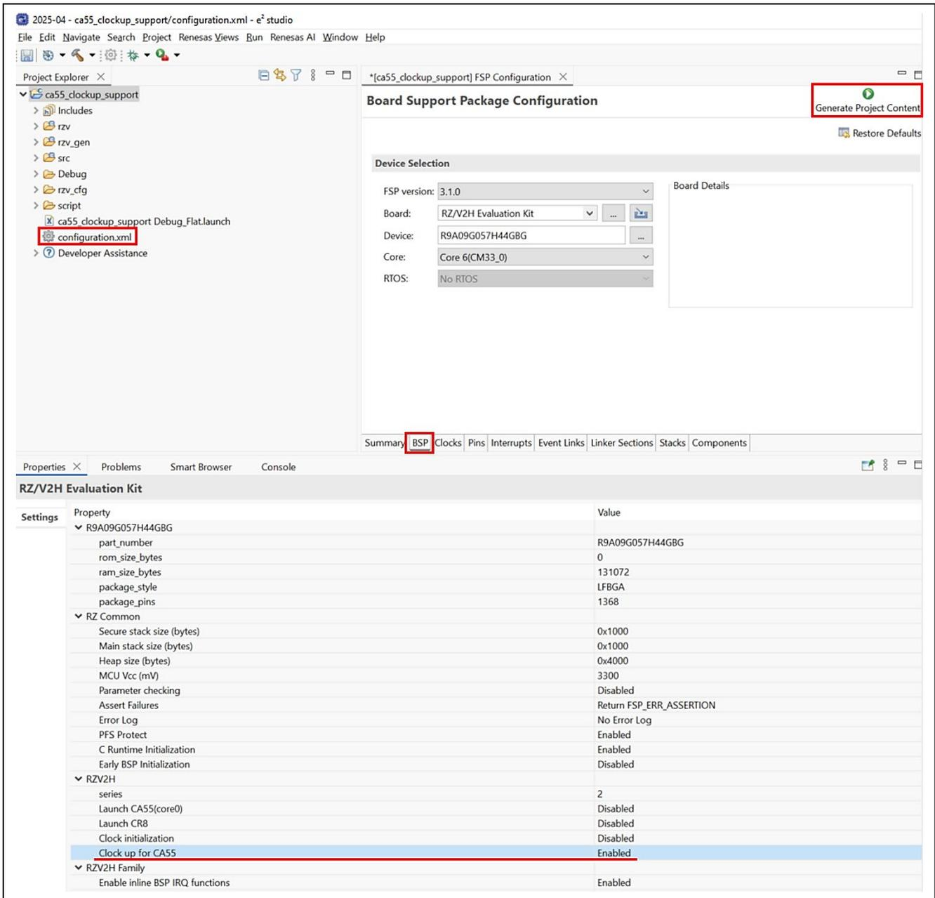
Figure 5-1. CM33 project setting for CA55 1.8GHz support (CA55 coldboot)
