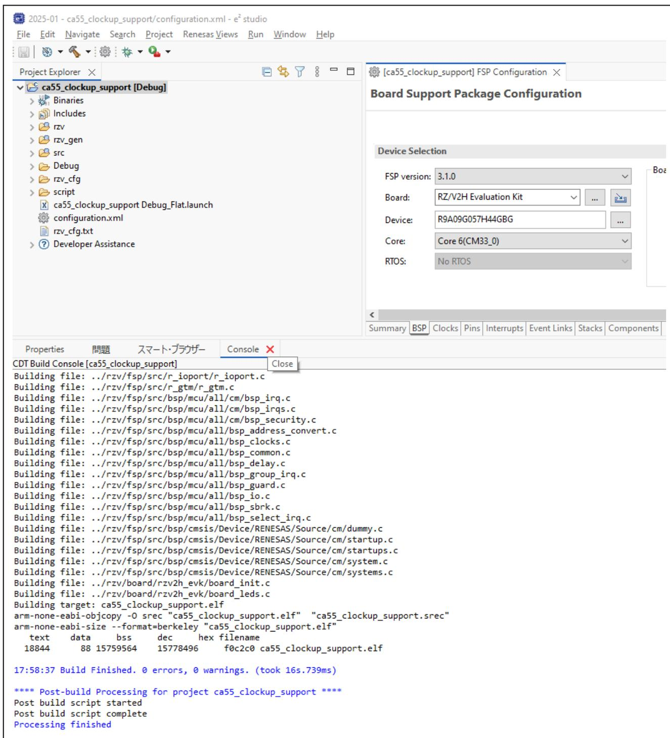
Figure 5-2. Build CM33 project for CA55 1.8GHz support
