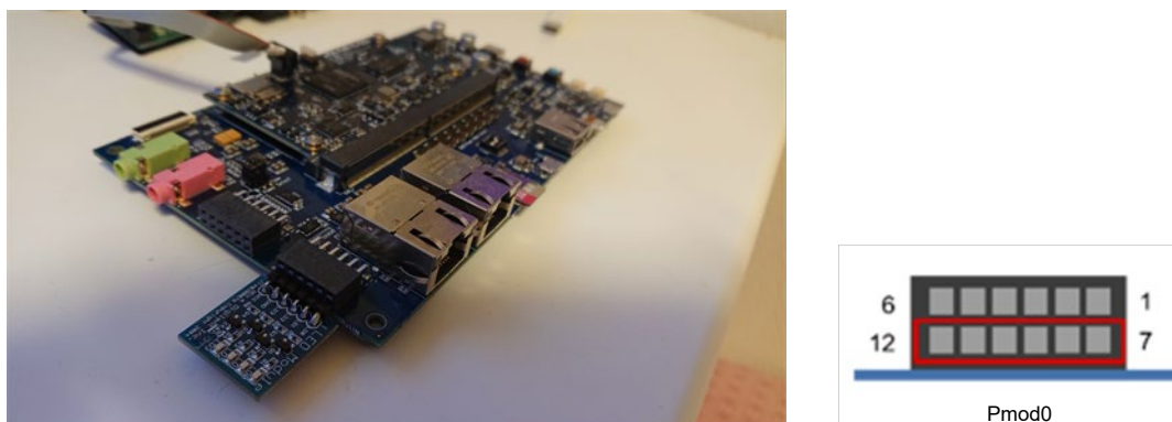
Figure 49: Connection Pmod LED module (410-076)
