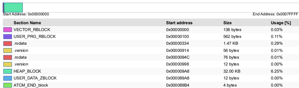
Figure 8.20. ATCM footprint of the CPU0 project (EWARM)
