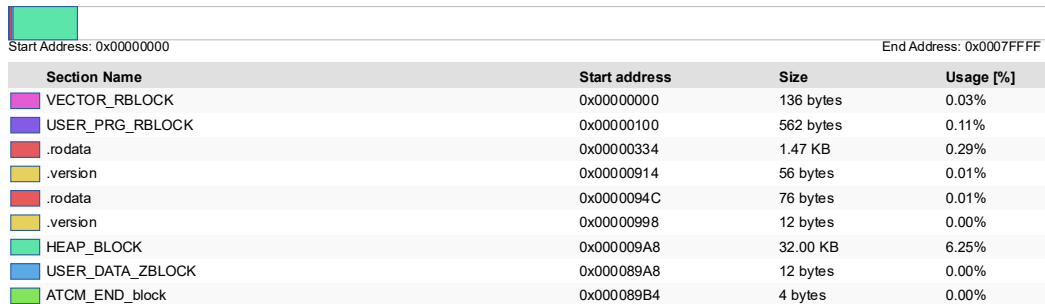
Figure 8.20. ATCM footprint of the CPU0 project (EWARM)
