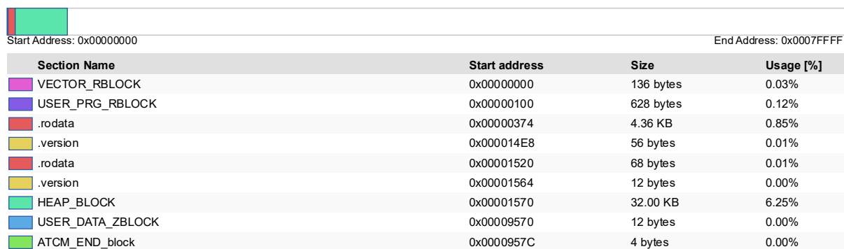
Figure 8.47. ATCM footprint of the CPU0 project (EWARM)
