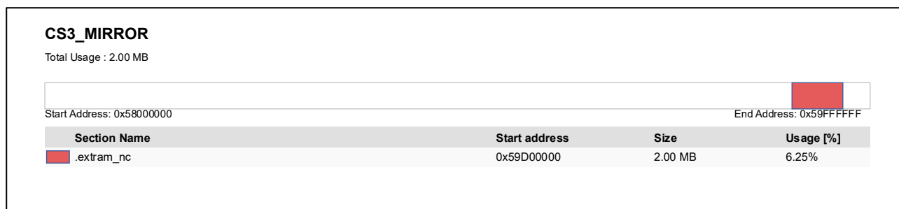
Figure 8.8. SDRAM MIRROR footprint of the xSPI Boot Single project (e 2 studio)
