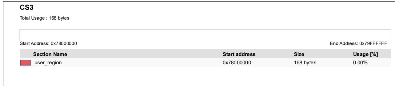
Figure 8.13. CS3 (SDRAM) footprint of the RZ/T2M Primary project (e 2 studio)
