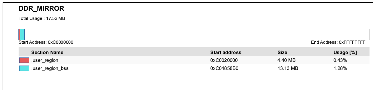
Figure 8.70. DDR_MIRROR footprint of the RZ/T2H, N2H (CA55_dual) Secondary project (e 2 studio)
