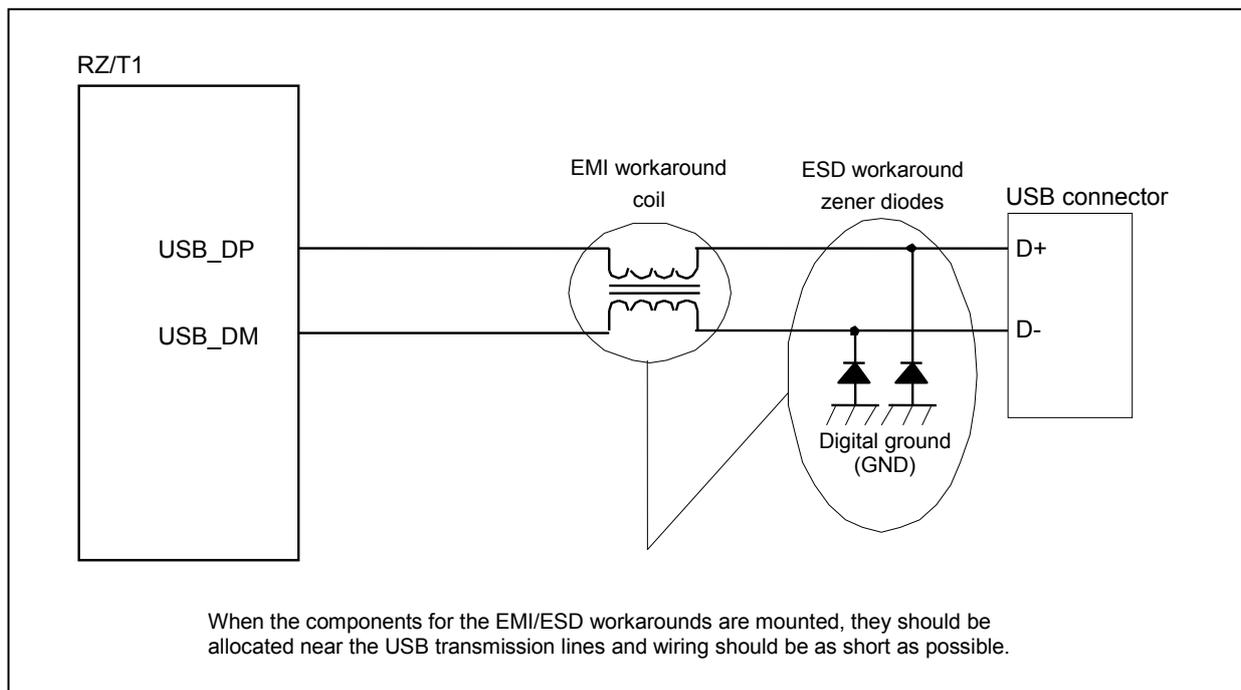
**Figure 6 Connection Example When Components for EMI/ESD Workarounds are Used**
