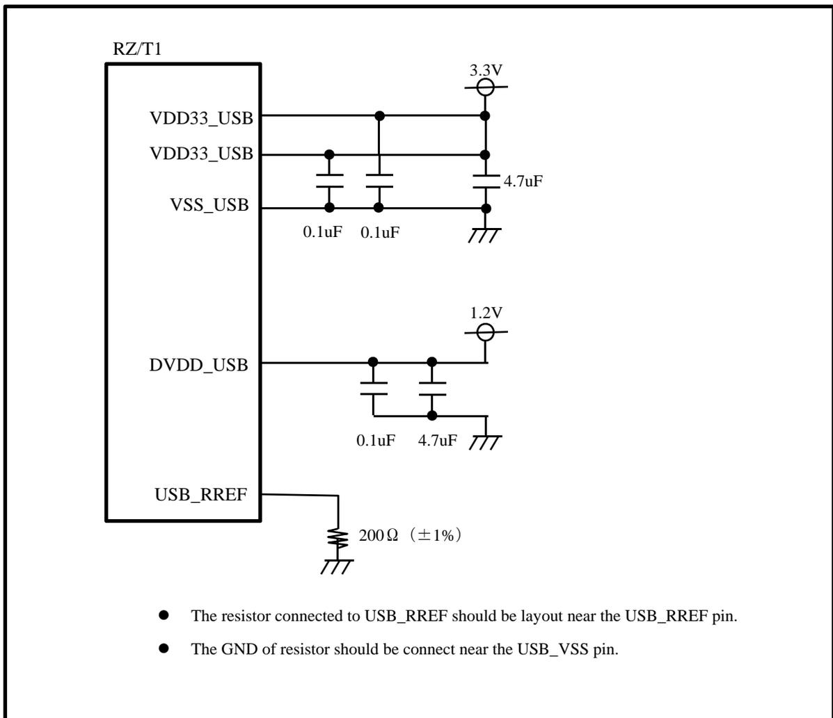
**Figure 3 Example of Decoupling Capacitor Allocation**
