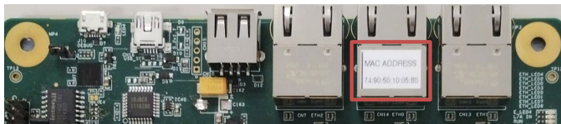
Fig. 5-1 MAC address pasted on CN14
