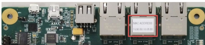
Fig. 5-1 MAC address pasted on CN14
