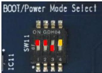
Change SW1 on the module to select micro SD card slot (SW1-1 ON, SW1-2 ON):
