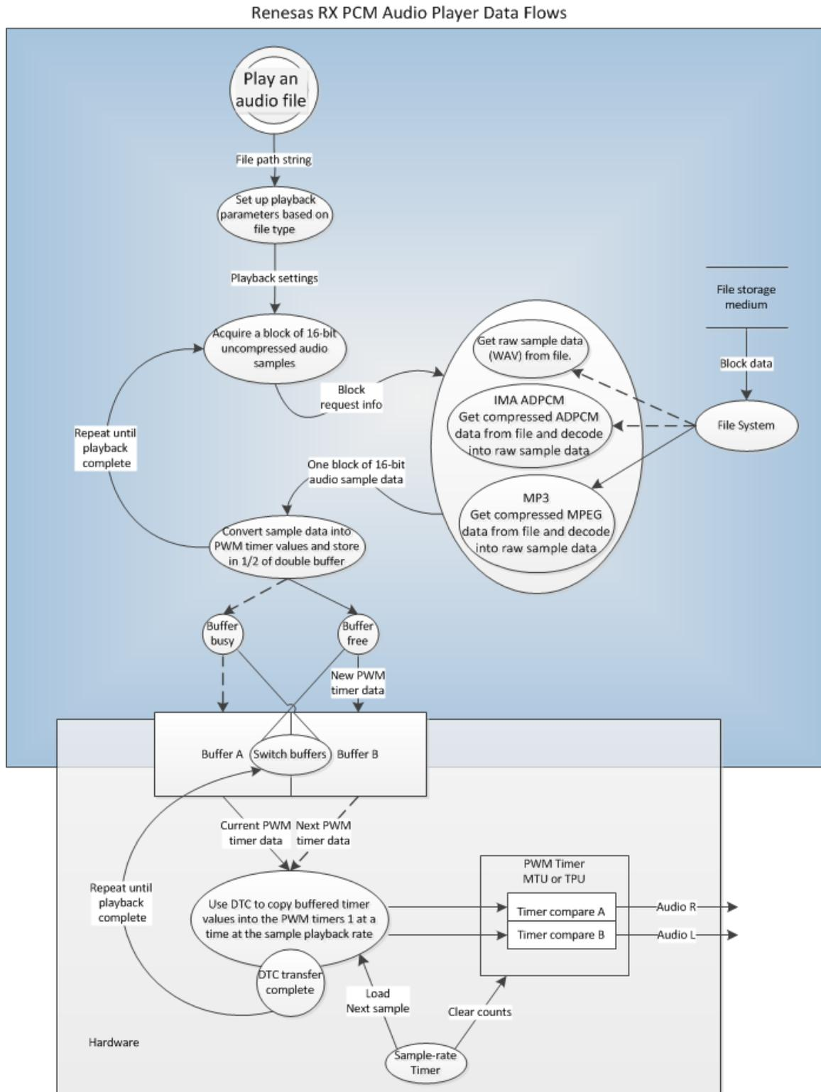
Figure 1 principle of operation
