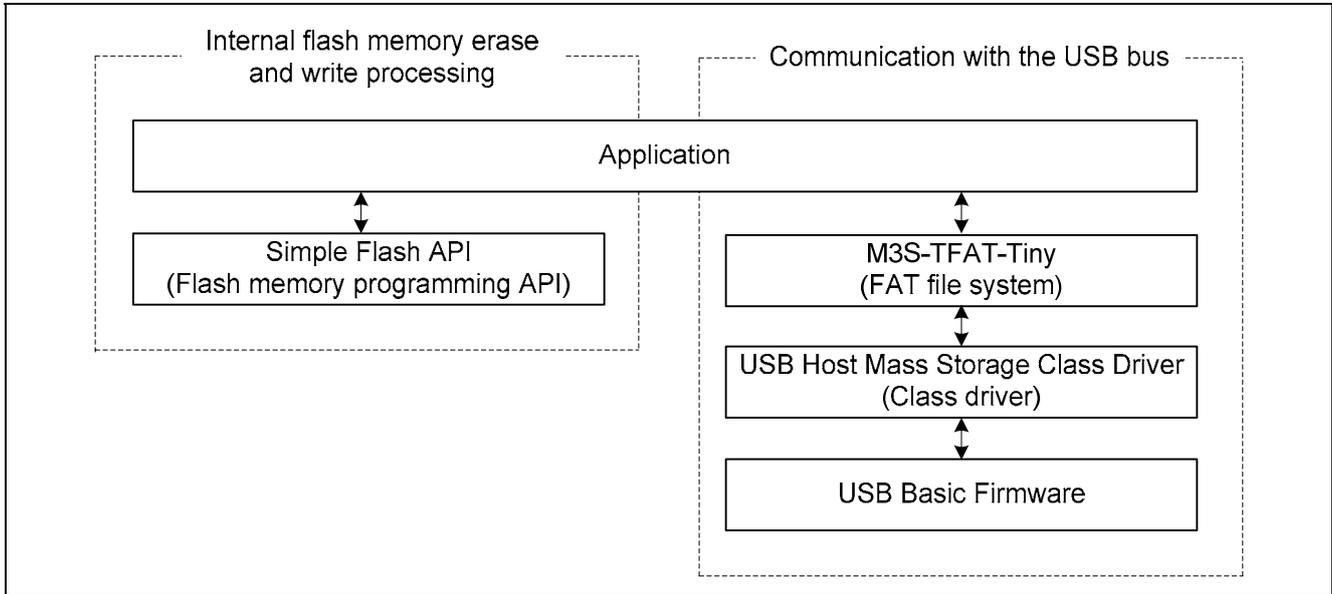
Figure 5.5 Software Structure of the Sample Code
