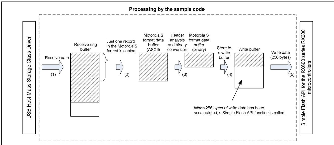
Figure 5.6 Data Flow During Write
