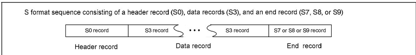
Figure 7.2 Record Structure Supported by the Sample Code
