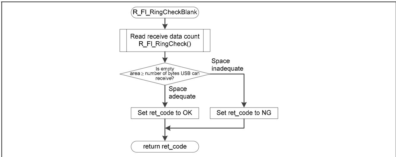
Figure 5.23 Check for Empty Space in Receive Data Storage Ring Buffer
