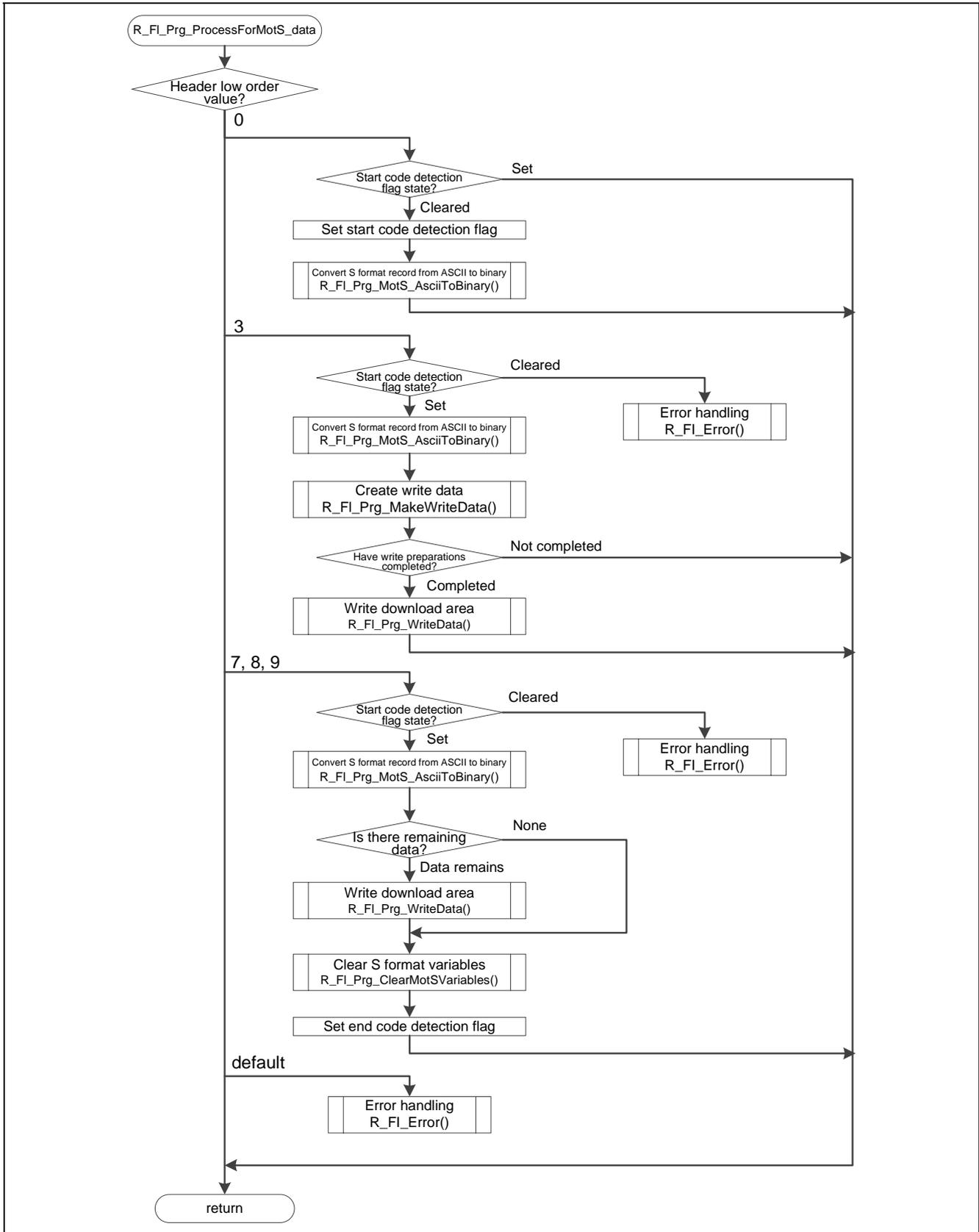
Figure 5.17 Format Header Analysis, Conversion to Binary, and Write Operations
