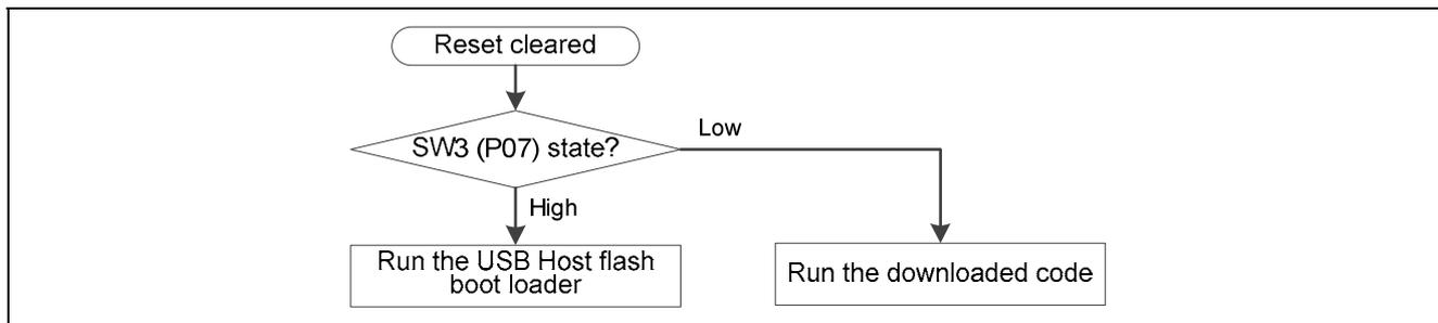
Figure 5.1 Operation After a Reset is Cleared
