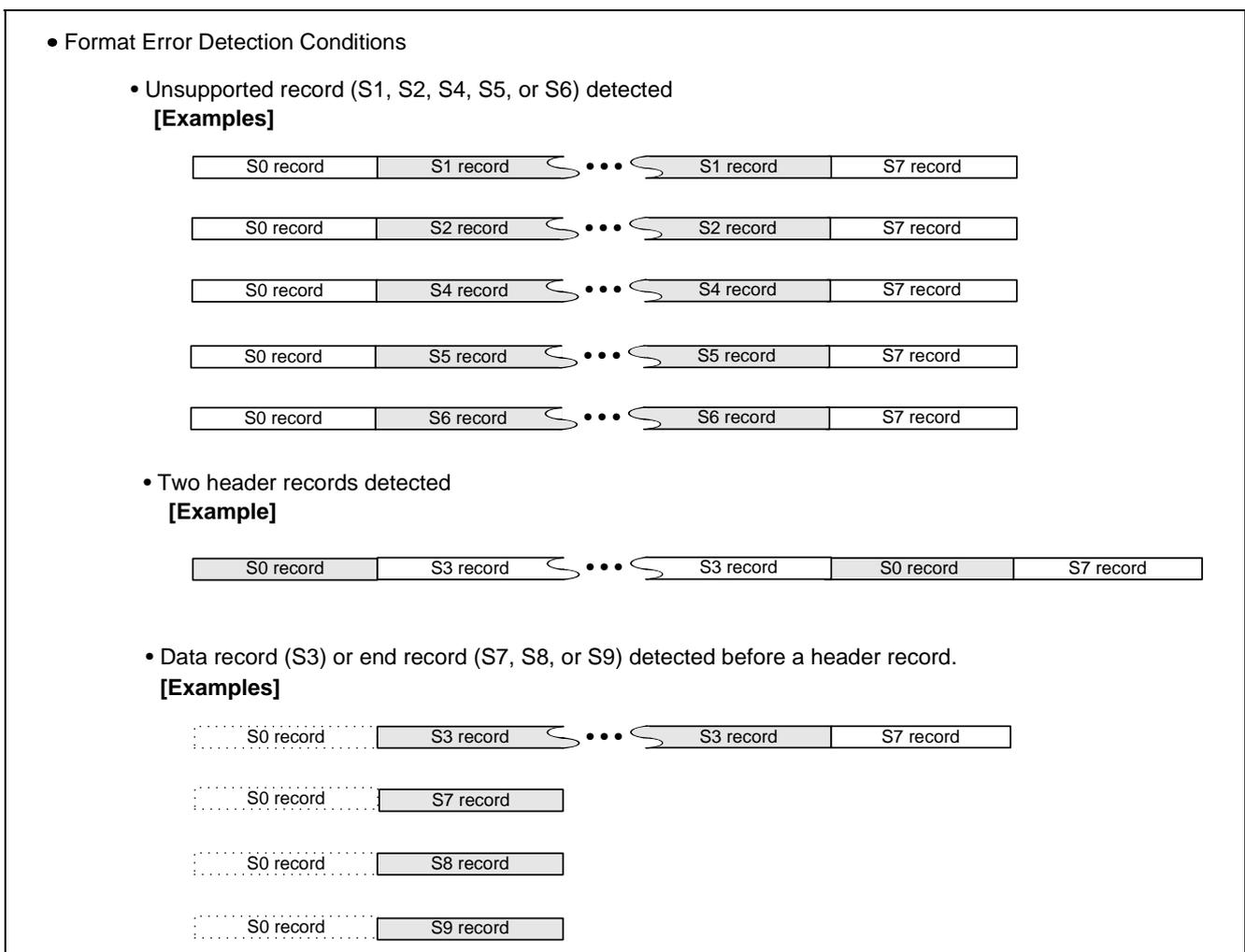
**Figure 7.3 Format Error Detection Conditions**
