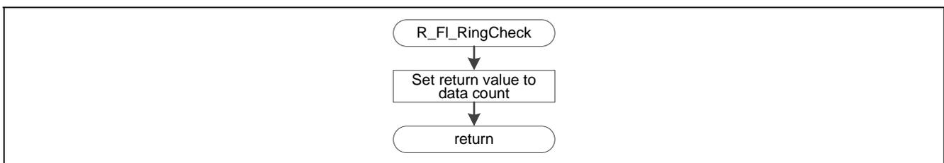
**Figure 5.28 Check Data Count in Receive Data Ring Buffer**
