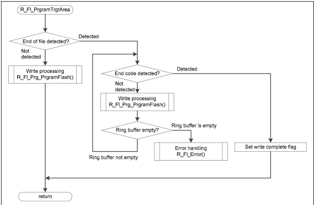
Figure 5.14 Write Processing
