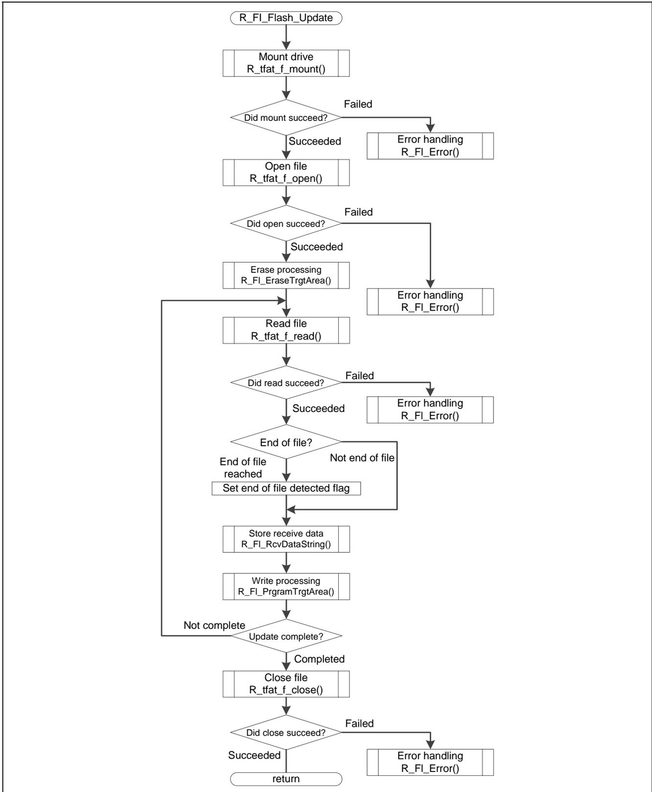
Figure 5.11 Main Write Processing
