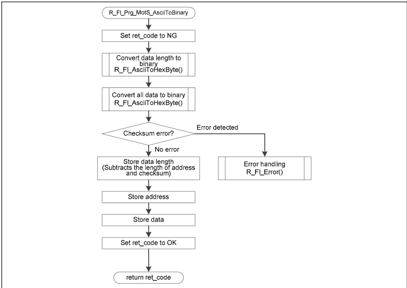
Figure 5.18 S Format Data ASCII to Binary Conversion
