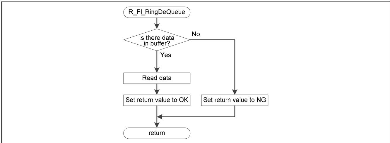
**Figure 5.27 Read Data from Receive Data Ring Buffer**
