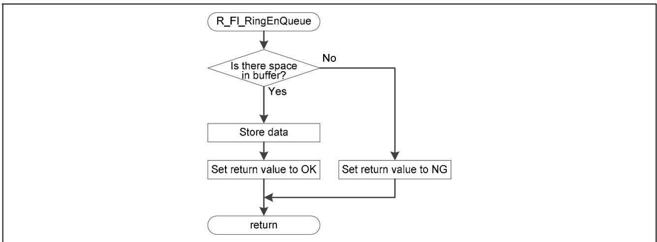
Figure 5.26 Store Data in Receive Data Ring Buffer
