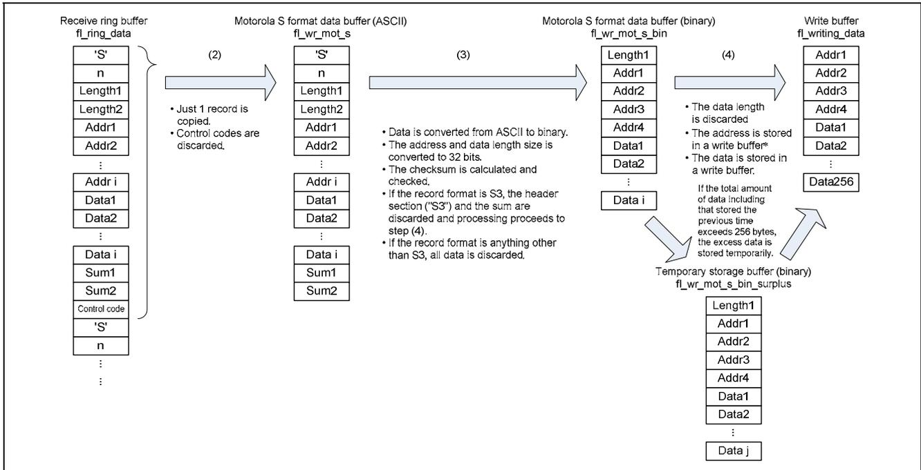
Figure 5.7 Data Structures Used for Writing
