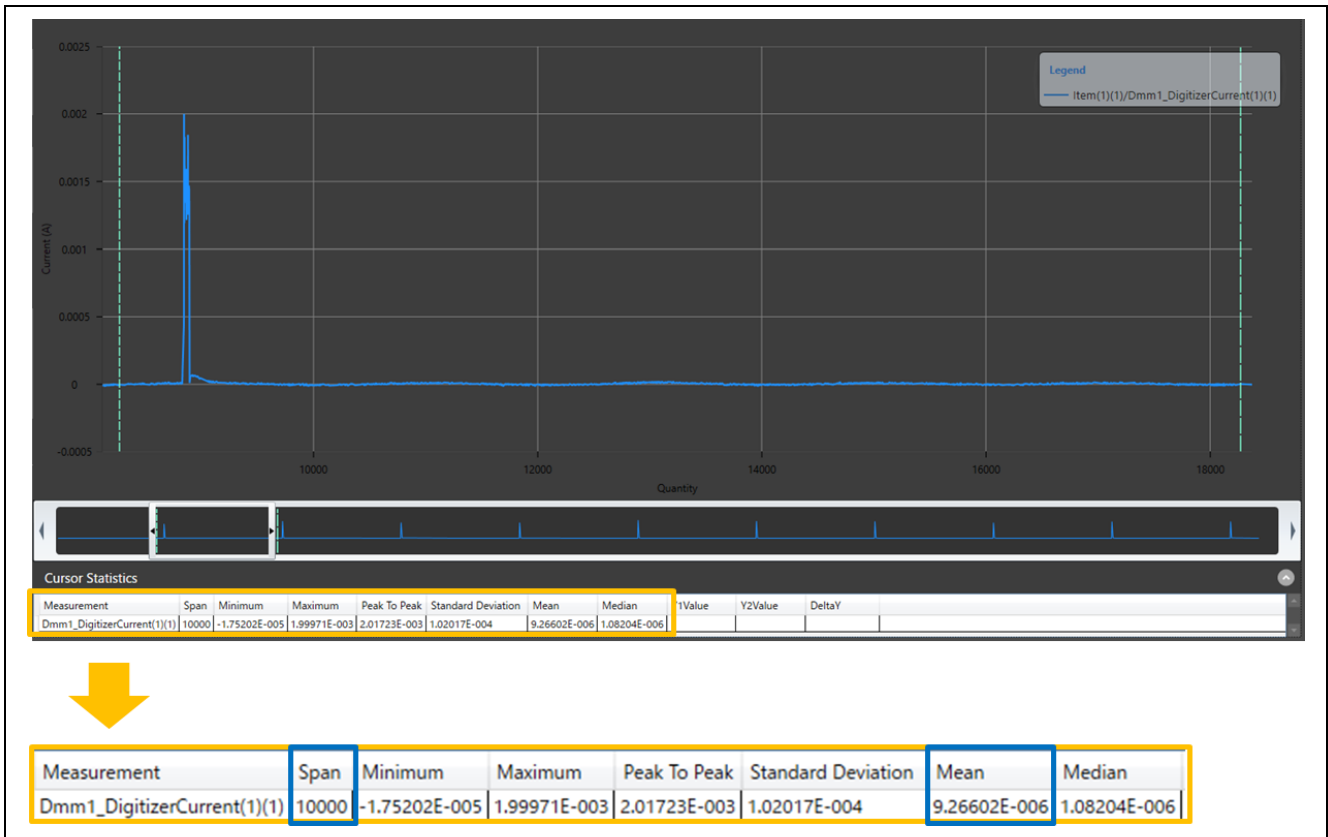
Figure 6.7 Average current of 100ms cycle in standby mode
