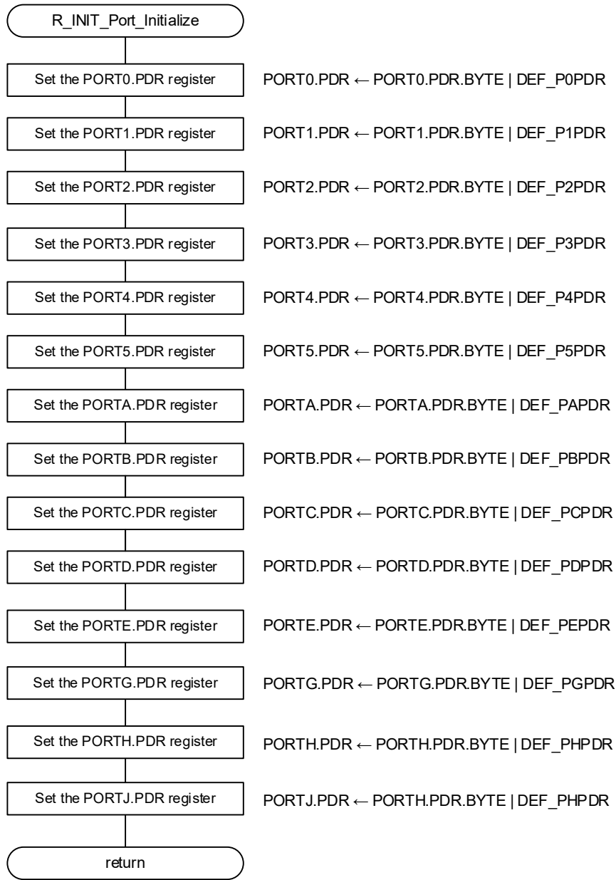
Figure 4.4 Nonexistent Port Initialization
