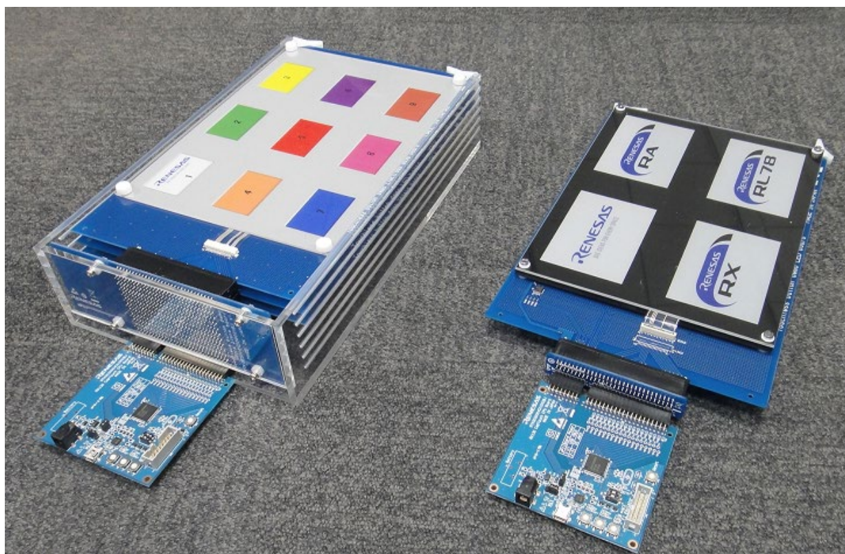
Figure 1.2 Touchless Button Electrode Board (Left: with housing, Right: without housing)
