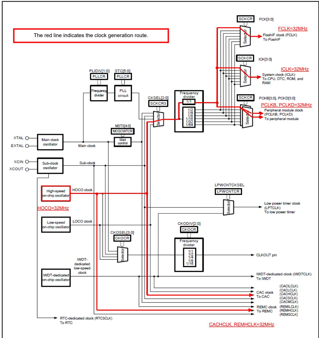
Figure 5-1: RX130 Clock generation block diagram
