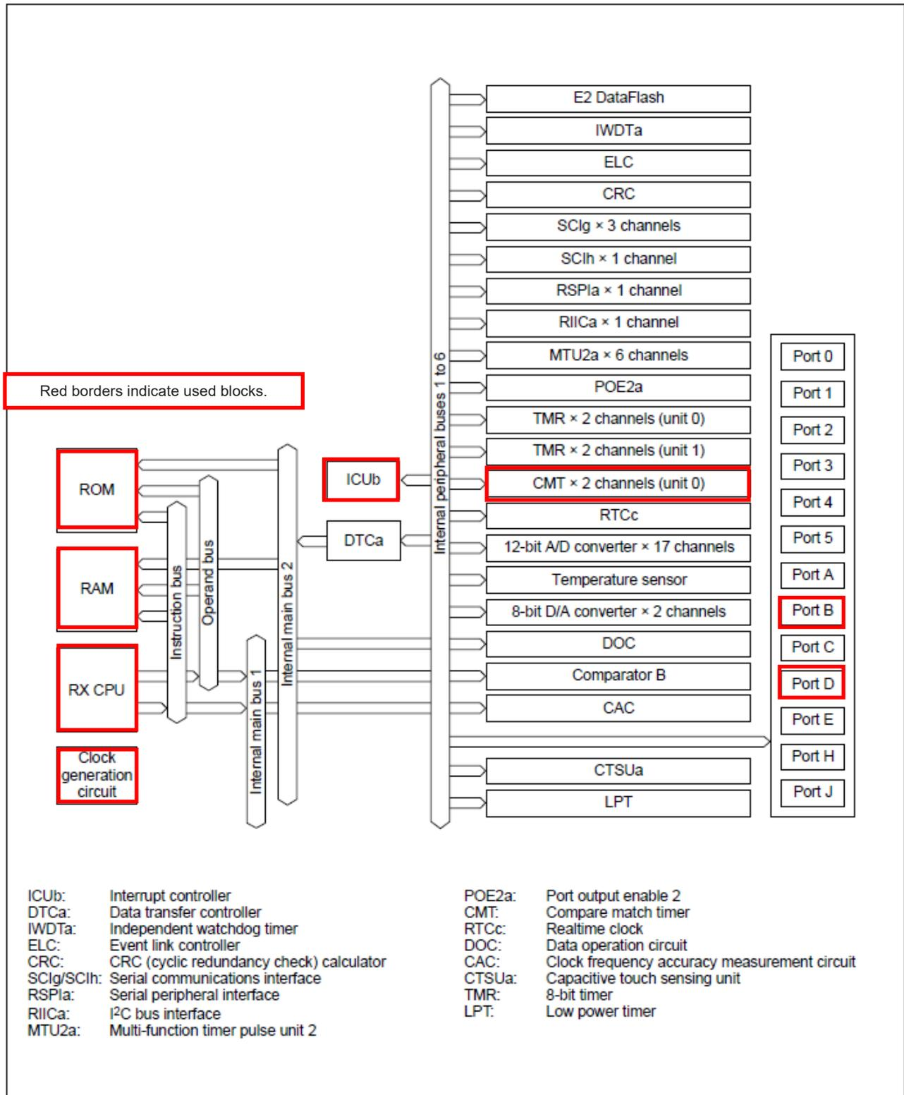
Figure 3-1: RX130 Internal block diagram
