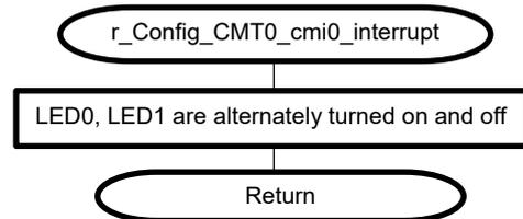
Figure 2-4: Timer interrupt operation flow
