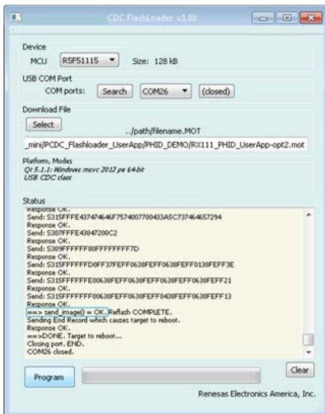
**Figure 2.** When the UserApp image is flashed successfully, “send\_image() = OK” is printed in the GUI text output.
