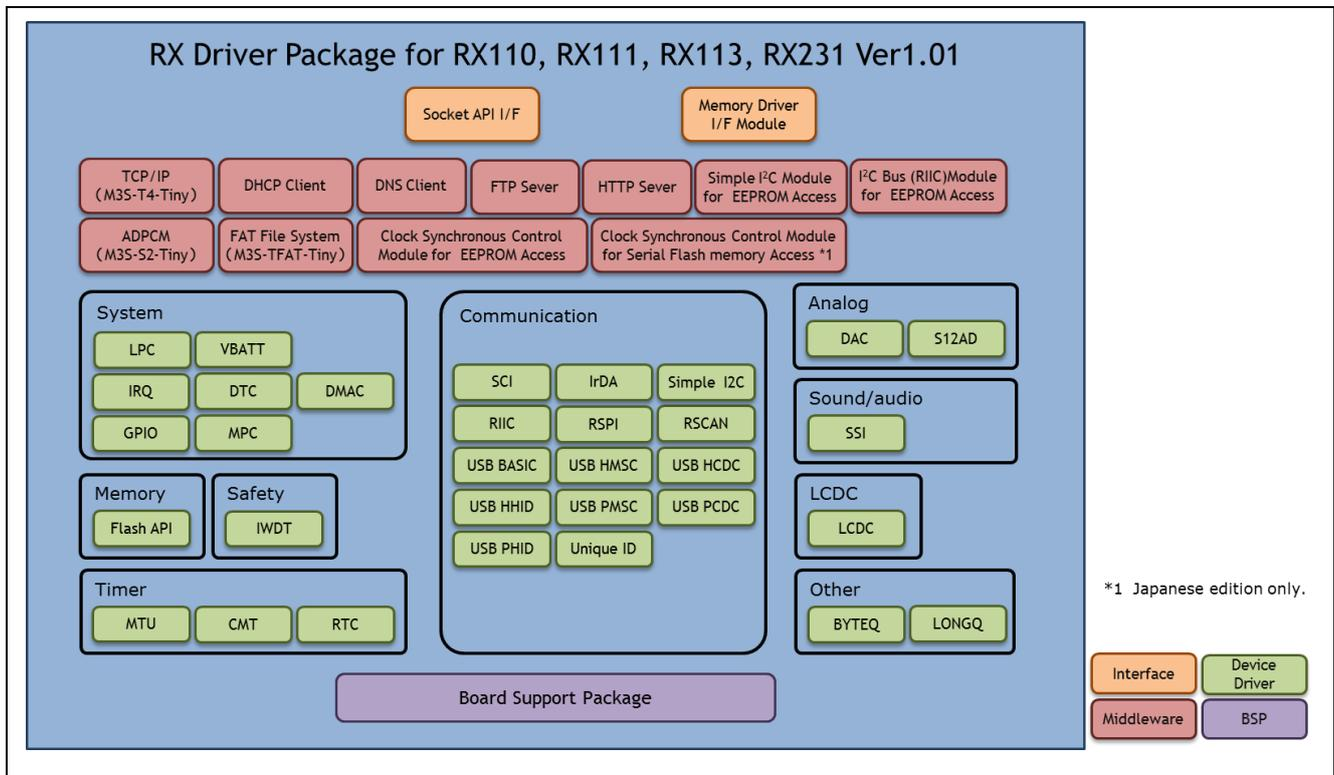
Figure 3-2 RX110, RX111, RX113, RX231 Group RX Driver Package FIT Module Structure
