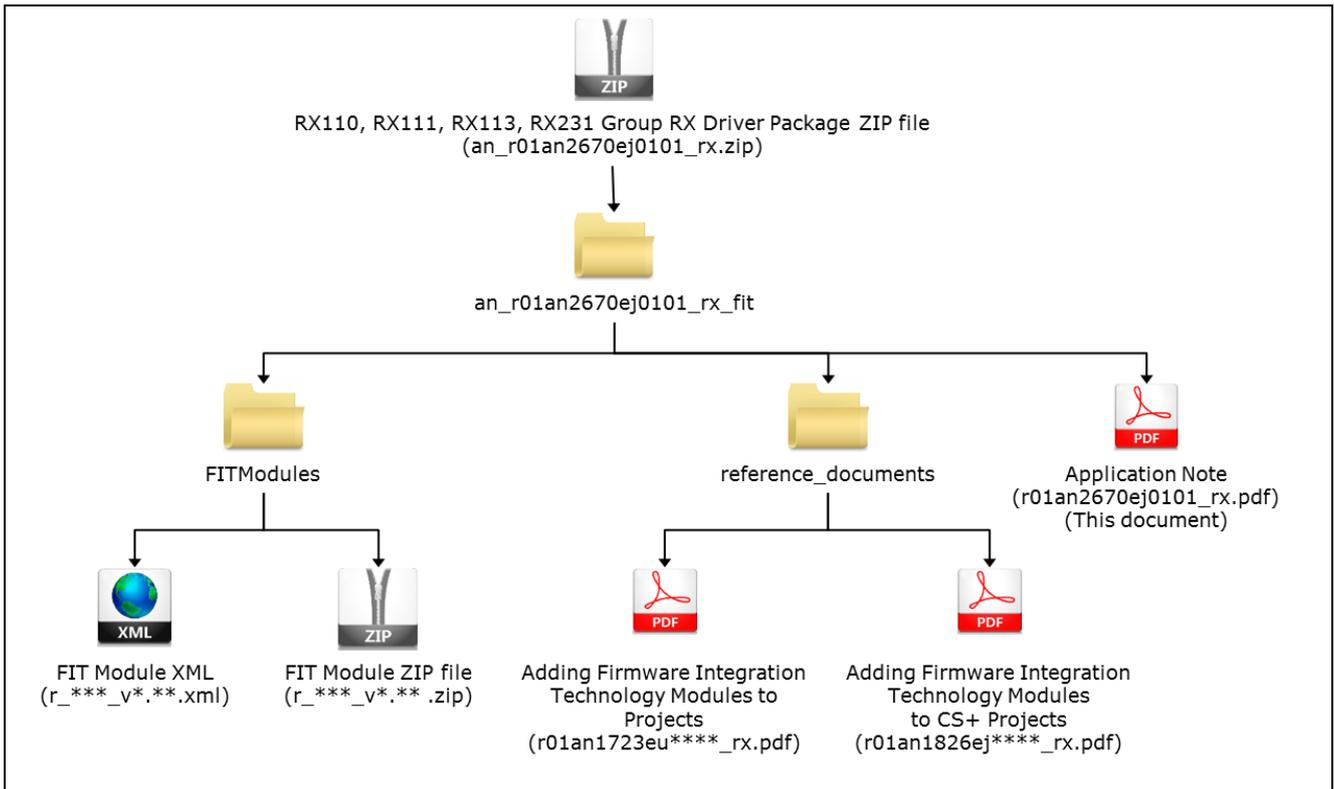
**Figure 3-1 Folder Structure of the RX110, RX111, RX113, RX231 Group RX Driver Package**
