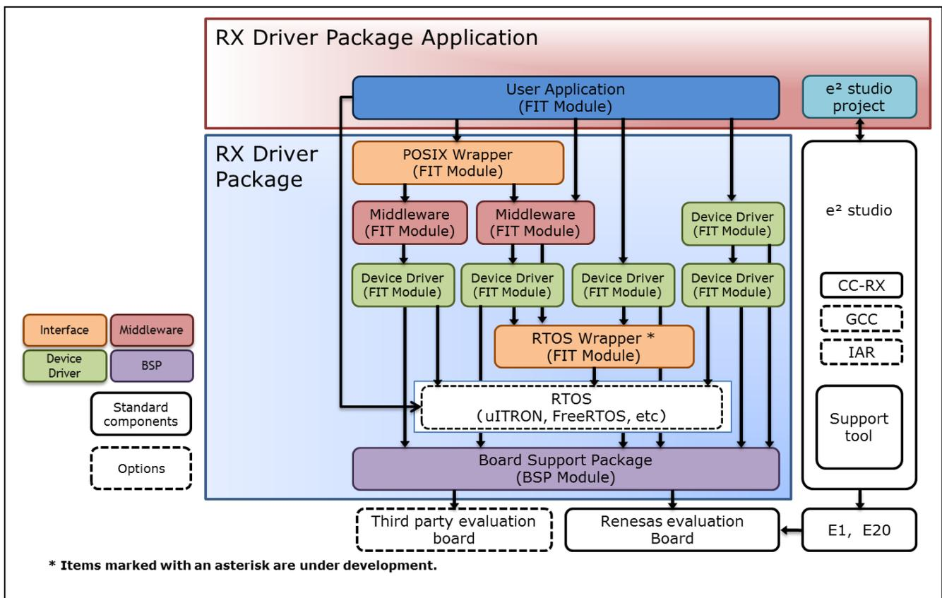
Figure 2-1 System Structure
