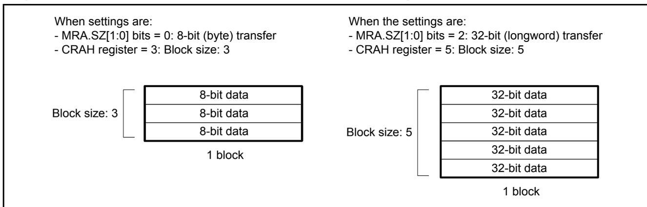
**Figure 4.1 Relation Between the MRA.SZ bit and the CRAH Register in Block Transfer Mode**
