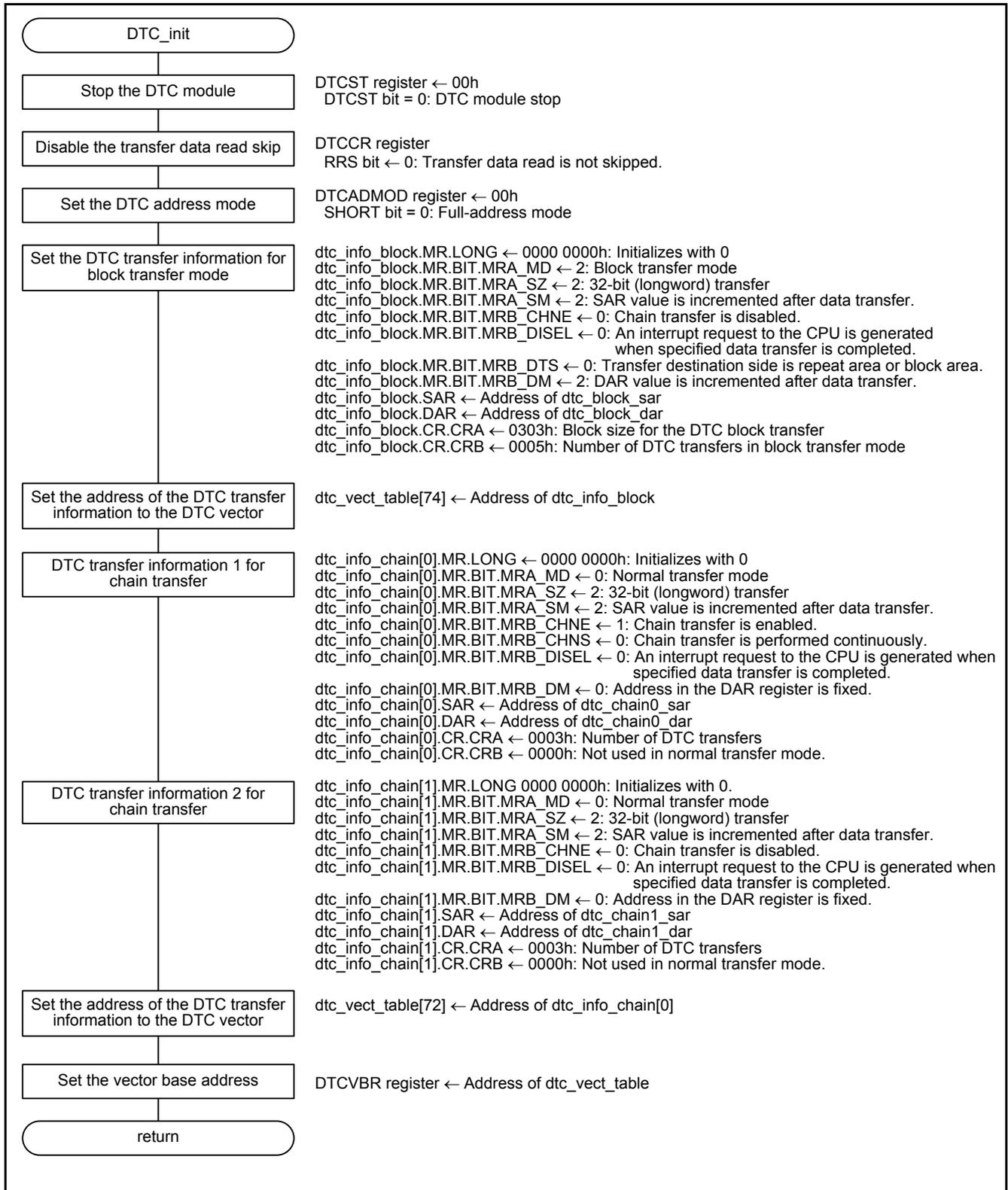
Figure 6.10 DTC Initialization
