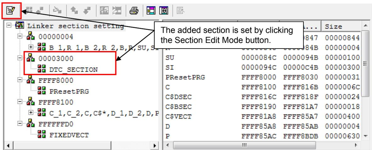
(4) Setting the start address for the DTC transfer information to the DTC vector table
