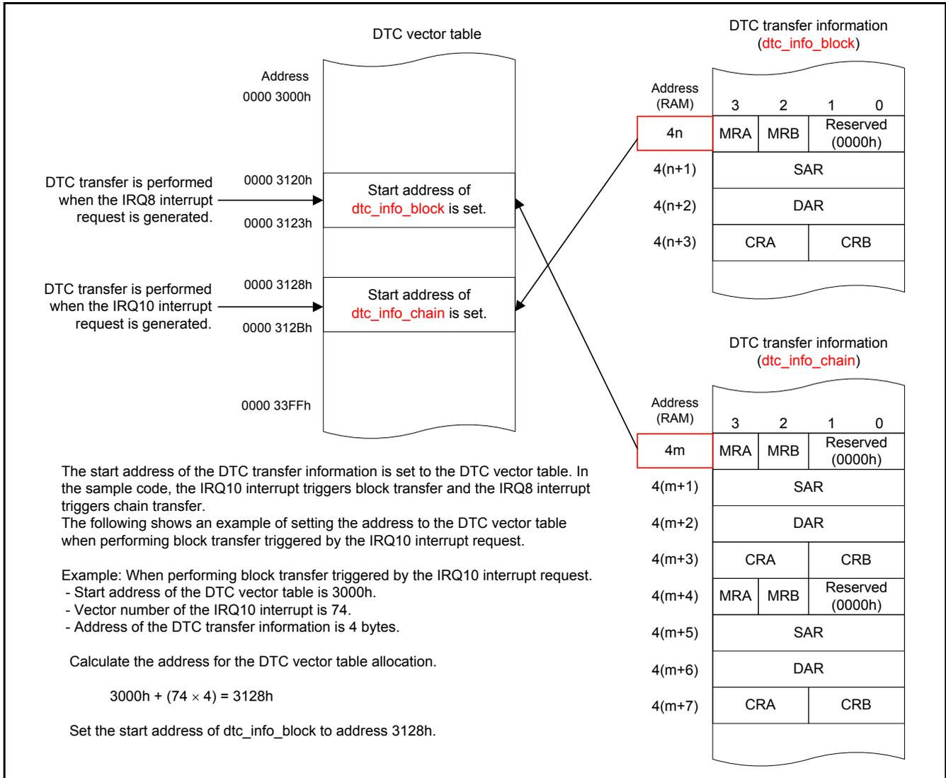
Figure 6.3 Setting the DTC Transfer Information to the DTC Vector Table
