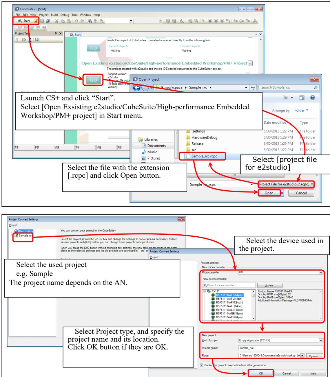
Figure 7-1 Using the e<sup>2</sup> studio project with CS+
