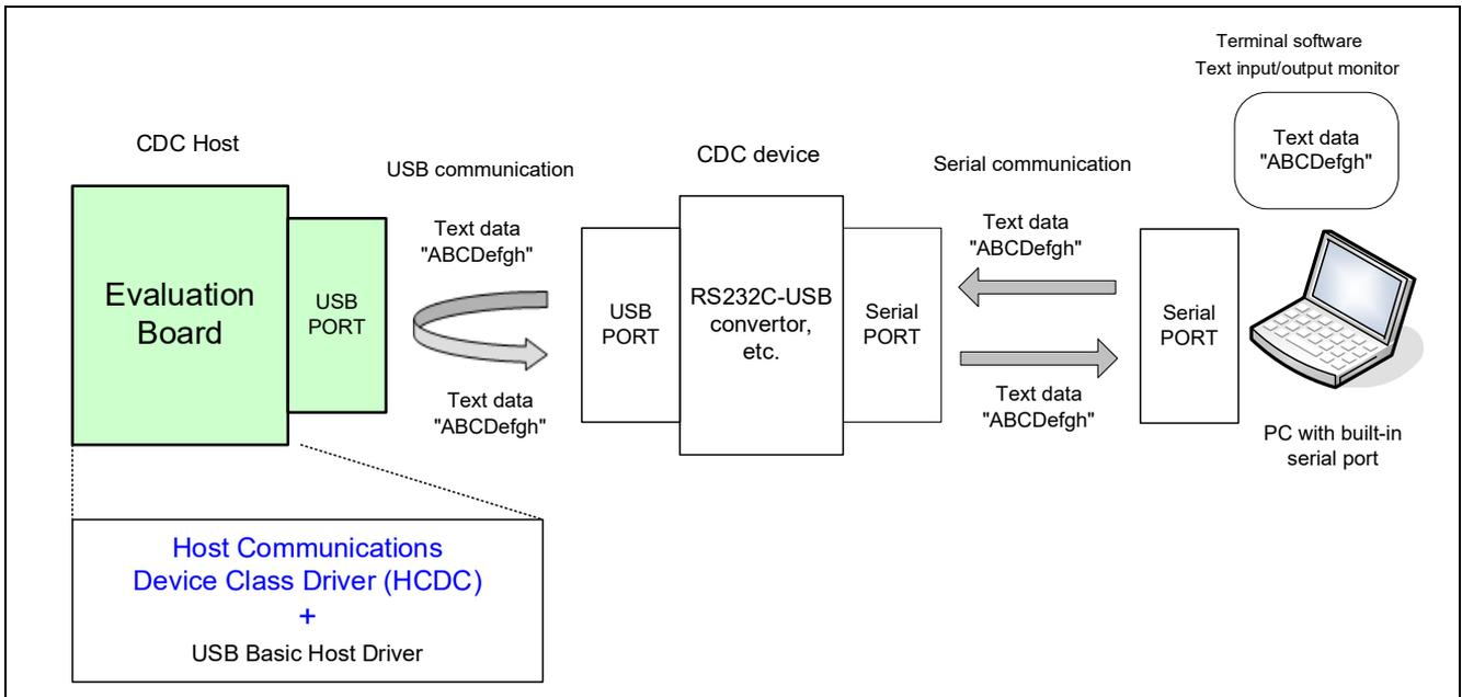
Figure 4-1 Data Transfer (Loopback) Image
