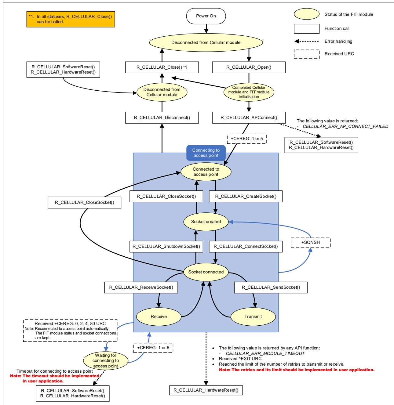
Figure 1.3 Status transitions of RYZ014A Cellular FIT module
