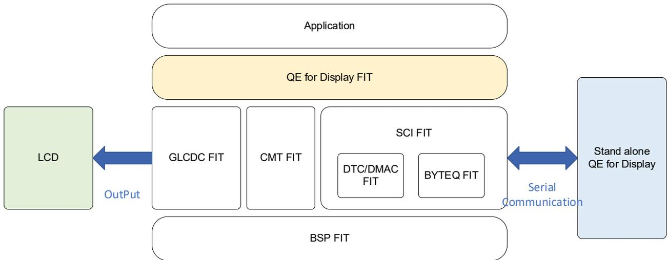
**Figure 1.1 Software Configuration**
