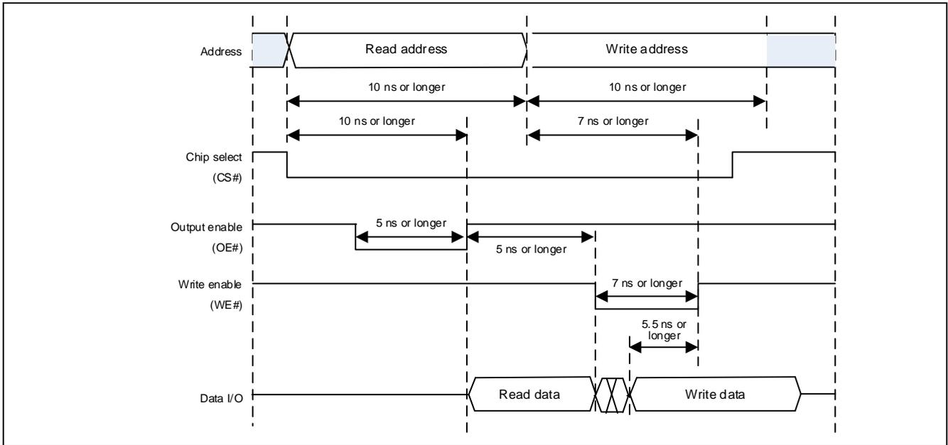
Figure 5.1 CY7C1061AV33 Control Timing for Read/Write Operations
