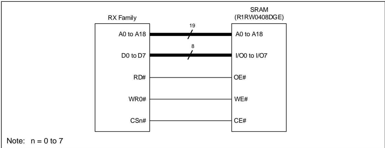
**Figure 6.2 Connection Example with 8-Bit Separate Bus**
