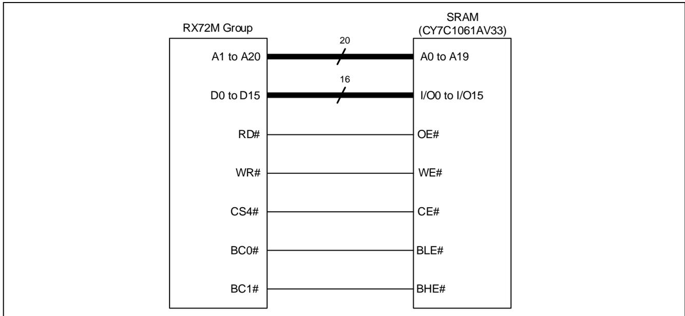
Figure 4.1 Connection Example with 16-Bit Separate Bus
