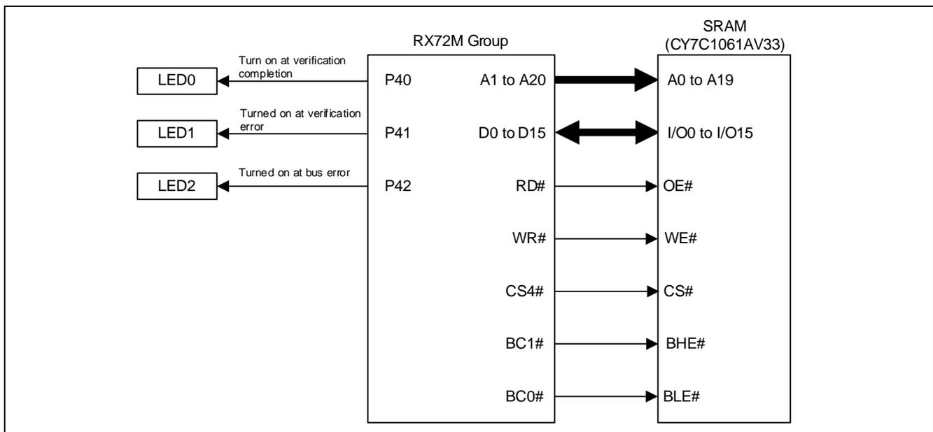
**Figure 3.1 Block Diagram**
