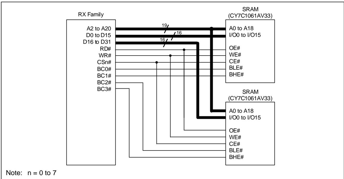
**Figure 6.3 Connection Example with 32-Bit Separate Bus**
