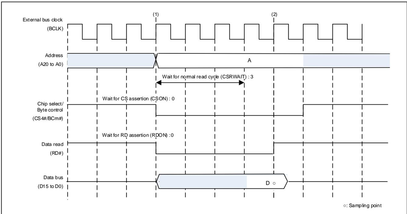
Figure 5.3 Bus Timing for Normal Read ( $m = 0$  and  $1$ )
