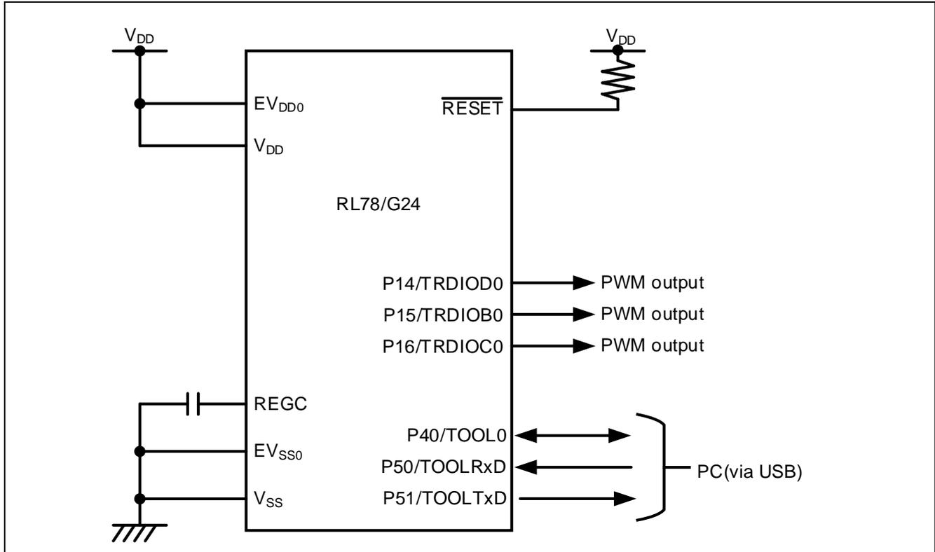
Note 1. This simplified circuit diagram was created to show an overview of connections only. When actually designing your circuit, make sure the design includes appropriate pin handling and meets electrical characteristic requirements (connect each input-only port to VDD or VSS through a resistor).
