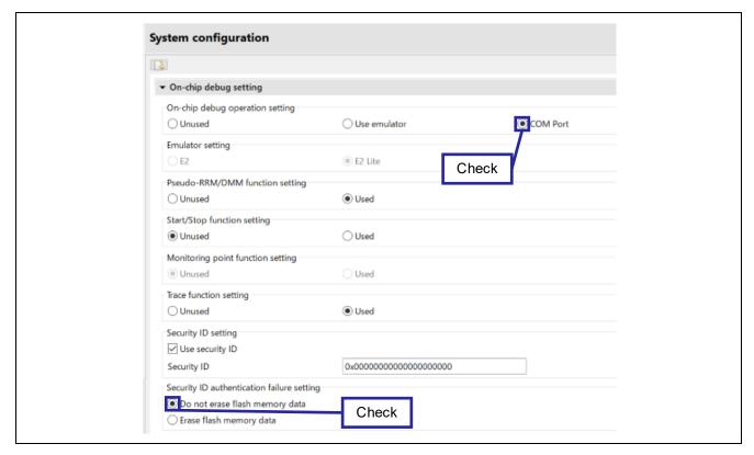
Figure 4-2 shows the system configurations used in this sample program for IAR.
