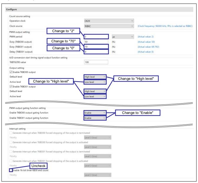
Note. The LED2 (green), controlled by the TKBO01 output, has a higher forward voltage (VF) than LED1 (red), which is controlled by the TKBO00 output. Therefore, the duty cycle is set to "70%" to increase the voltage applied to the LED by setting a higher duty cycle.
