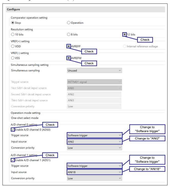
Figure 4-6 Configuration of A/D Converter (2/2)
