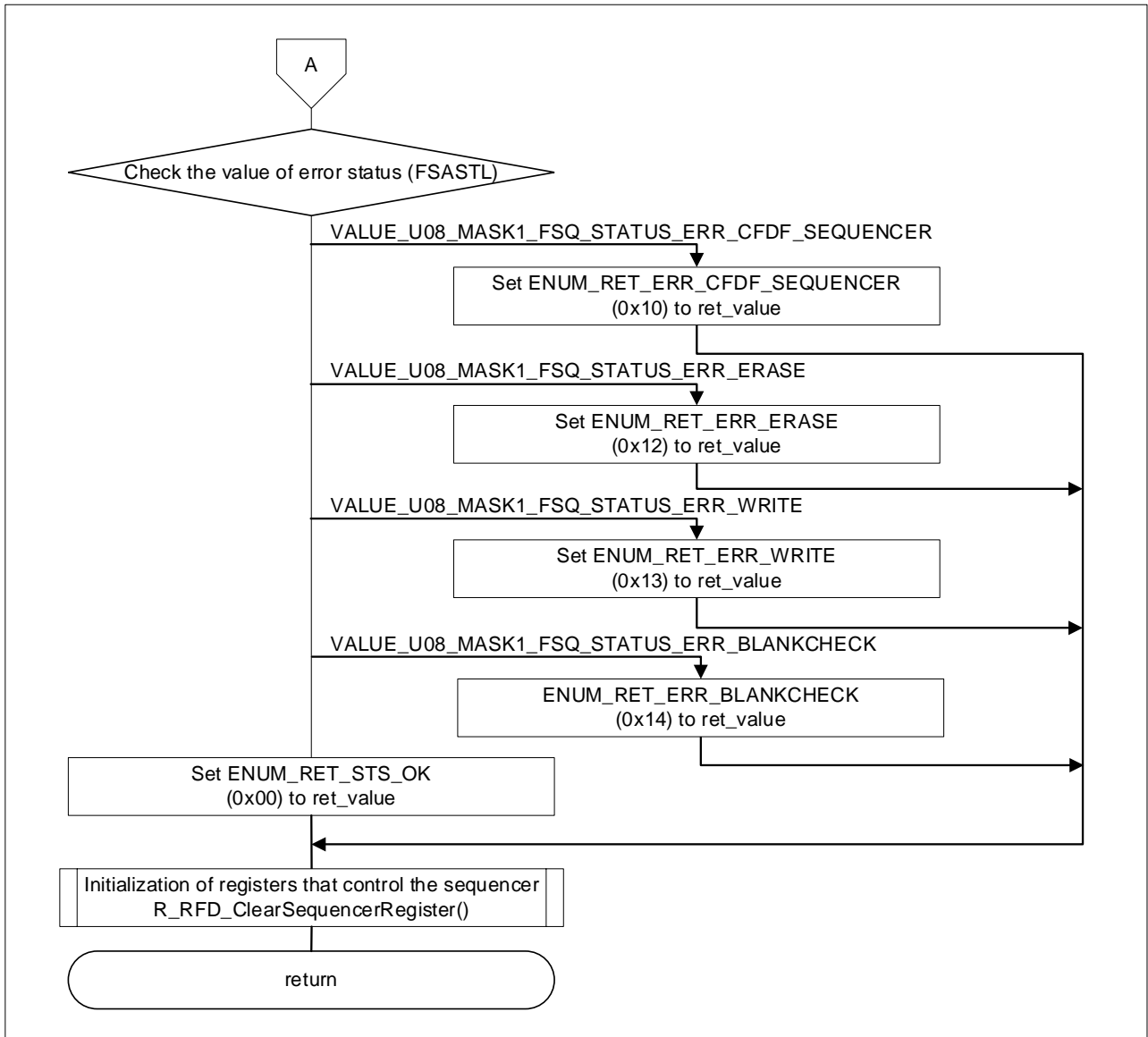
Figure 4-15 Sequence end processing for the code flash memory (2/2)
