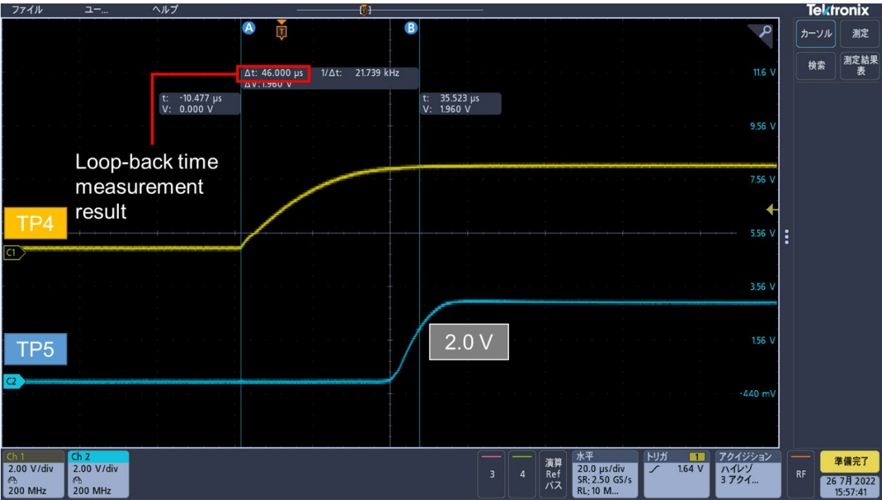
Figure 4-21 Loop-back time measurement results
