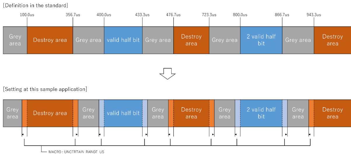
Figure 4-14 Definition in the standard for Multi-master Transmitter and the sample application setting (starting at an edge inside of a logical bit)
