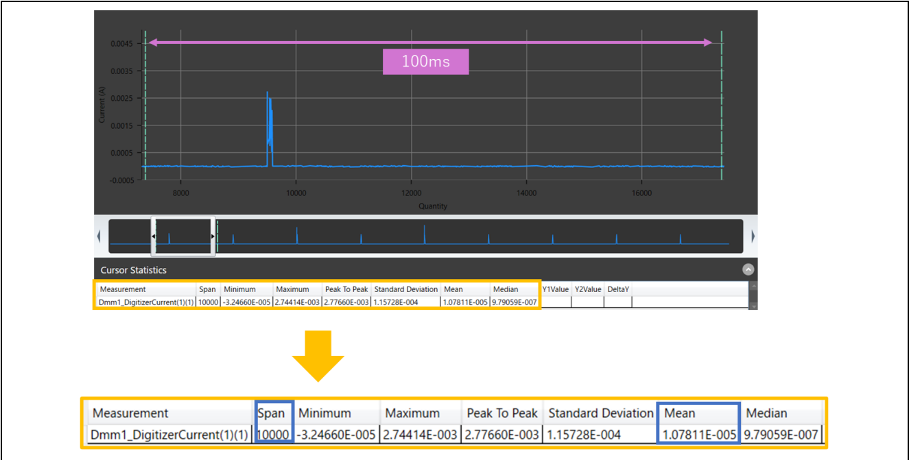
Figure 10.3 Current consumption result by the KEITHLEY/KickStart (touch measurement using SMS)
