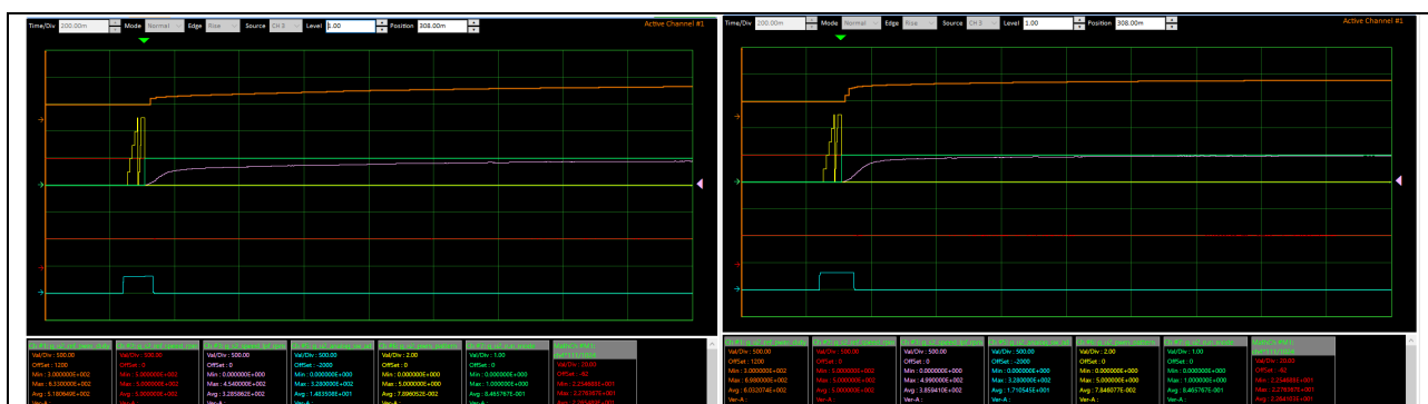
Figure 4-6 – Comparison of response by changing g_s2_spd_err_band (left : 2000, right 1000)
