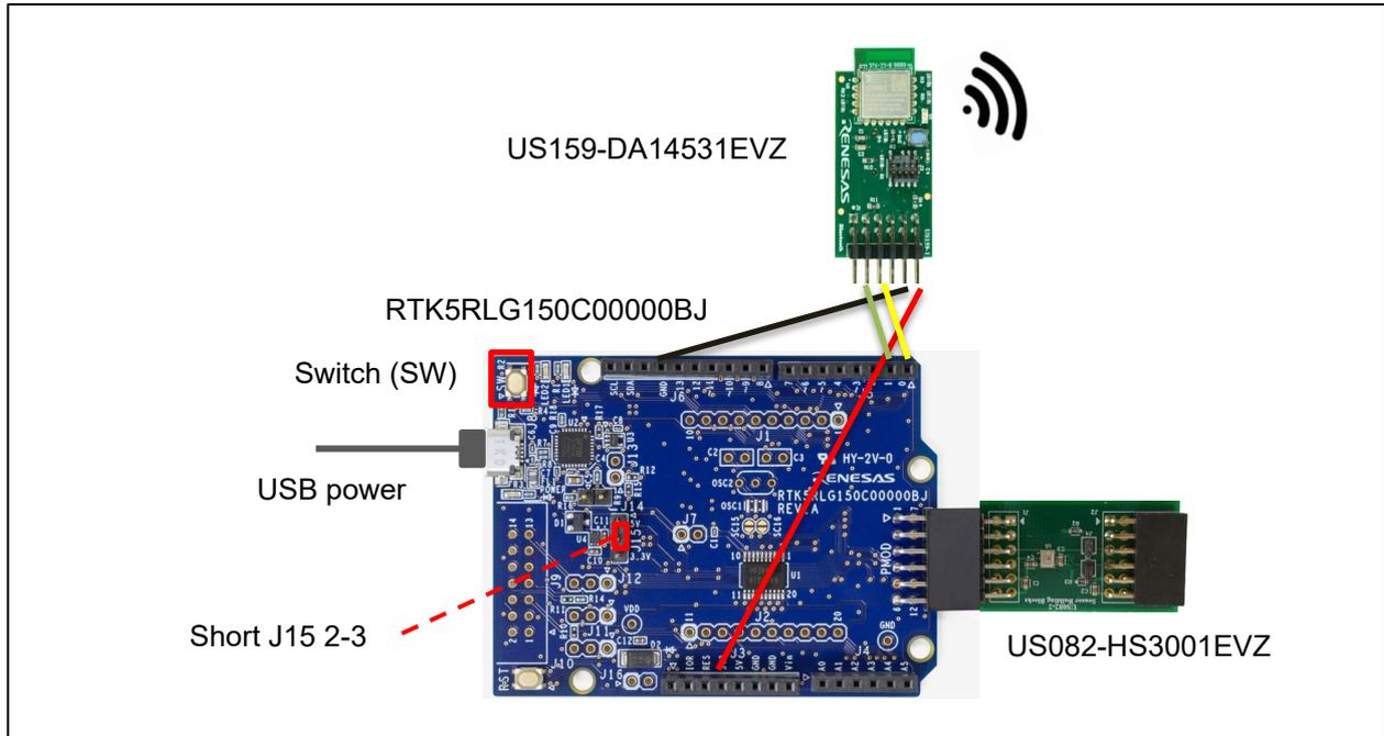
Table 6-2 Pins to which RTK5RLG150C0000BJ and US159-DA14531EVZ Connect
