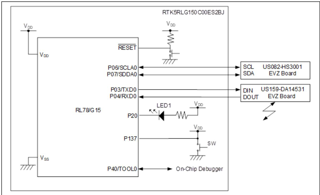
Note 1. This schematic circuit diagram is simplified to show the outline of connections. When creating circuits, design them so that they meet electrical characteristics by properly performing pin processing. (Connect input-only ports to V<sub>DD</sub> or V<sub>SS</sub> individually through a resistor.)
