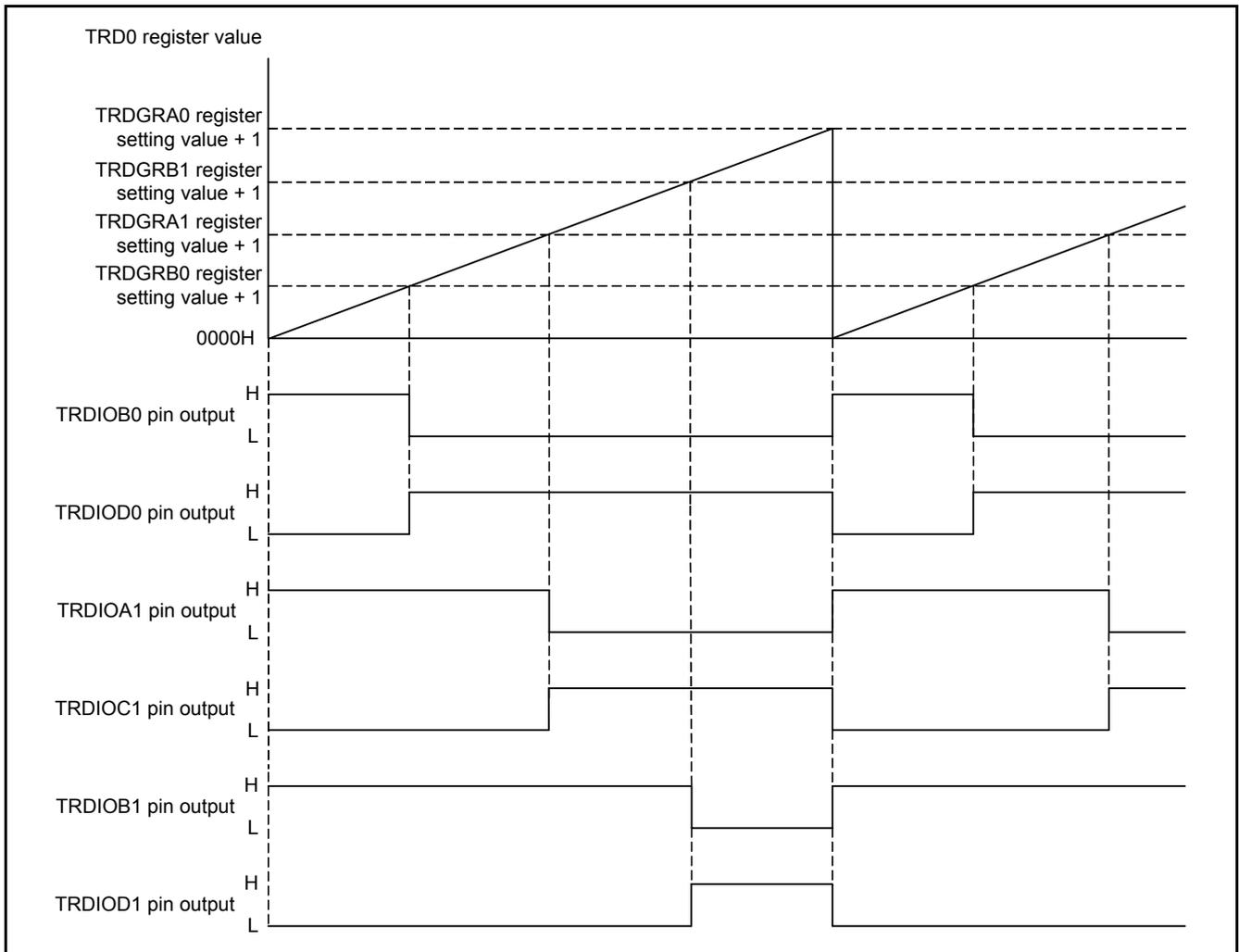
**Figure 1.1 Output Waveform of Reset Synchronous PWM**
