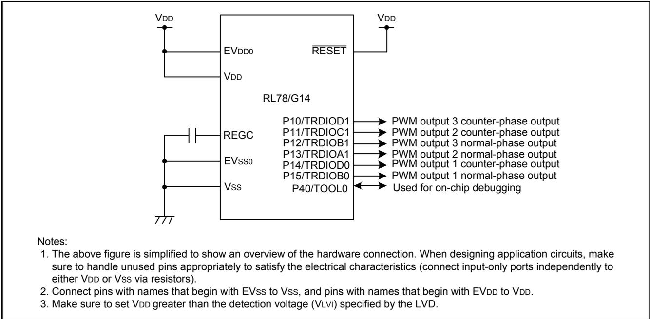
Figure 3.1 Hardware Configuration
