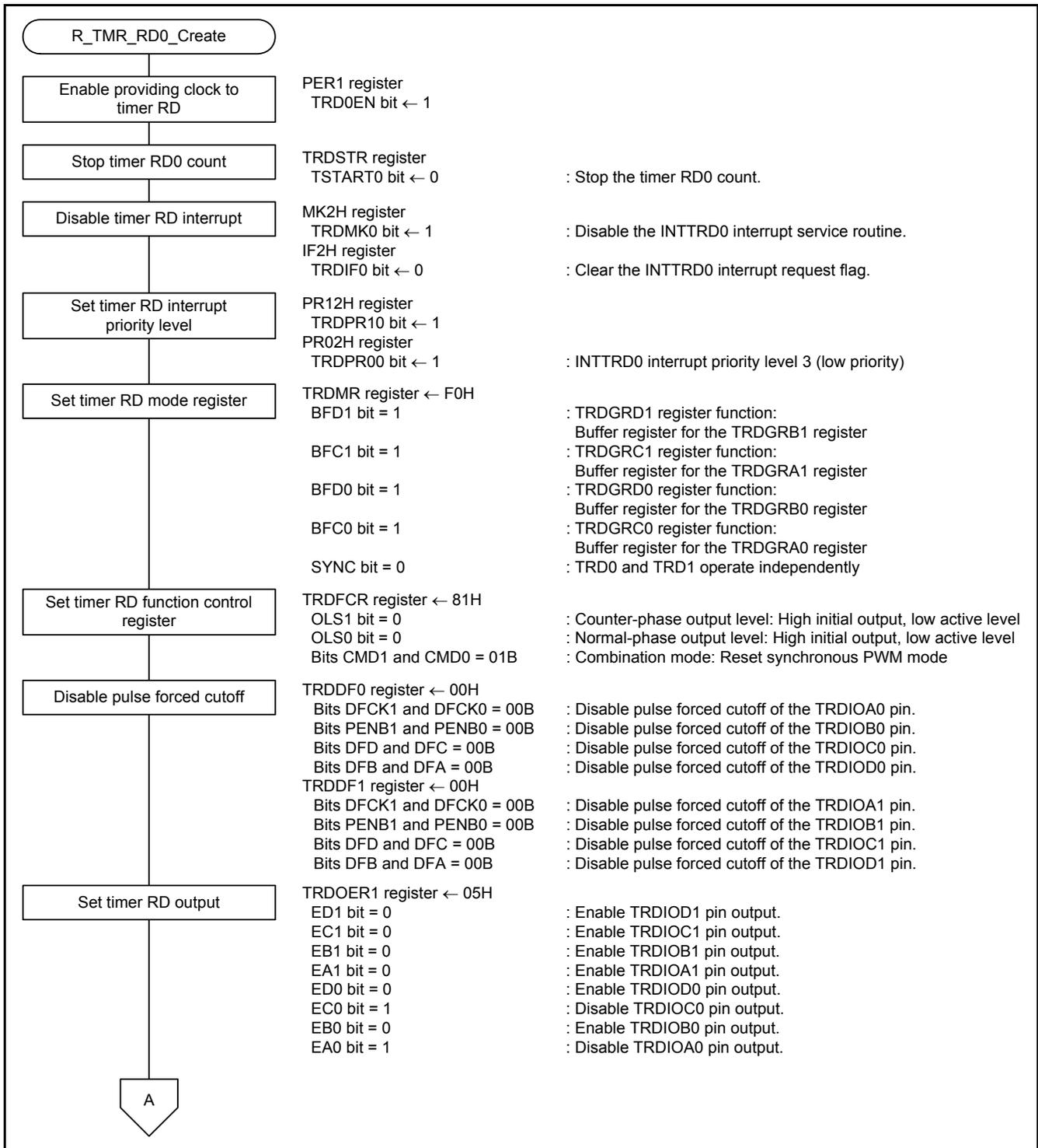
Figure 4.6 Initial Setting of Timer RD (1/2)
