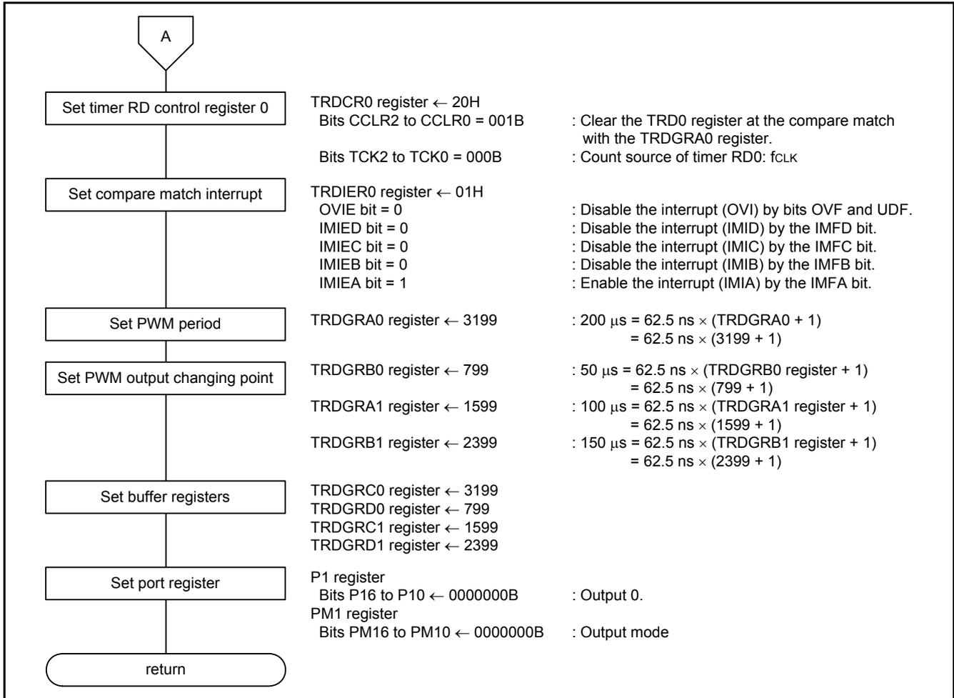
Figure 4.7 Initial Setting of Timer RD (2/2)
