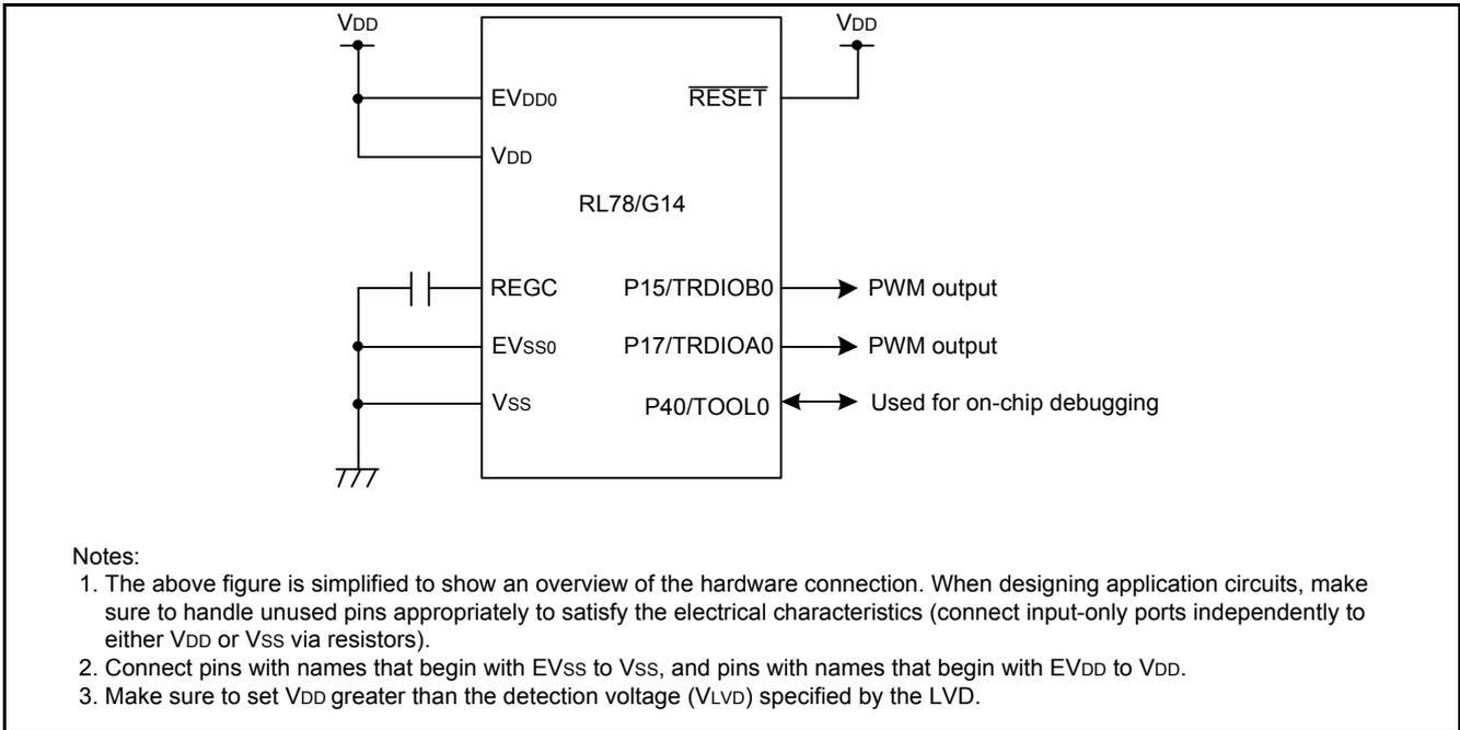
Figure 3.1 Hardware Configuration
