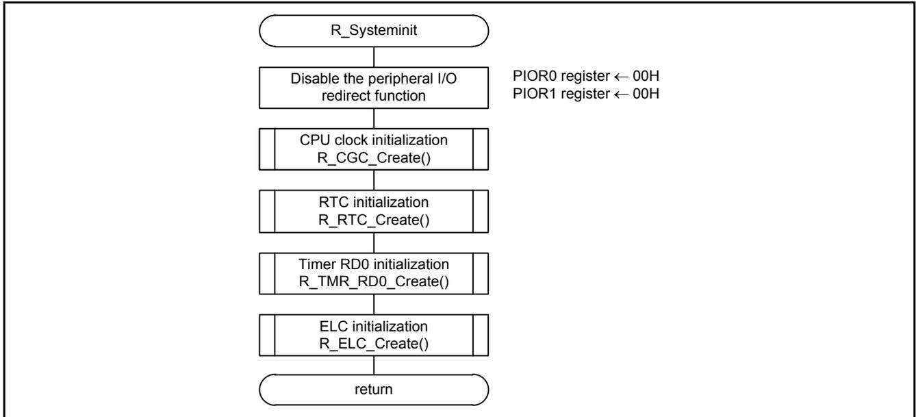
Figure 4.4 Peripheral Function Initialization
