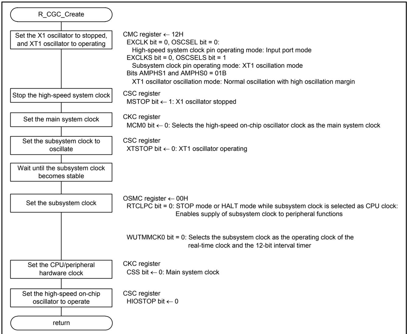
Figure 4.5 CPU Clock Initialization
