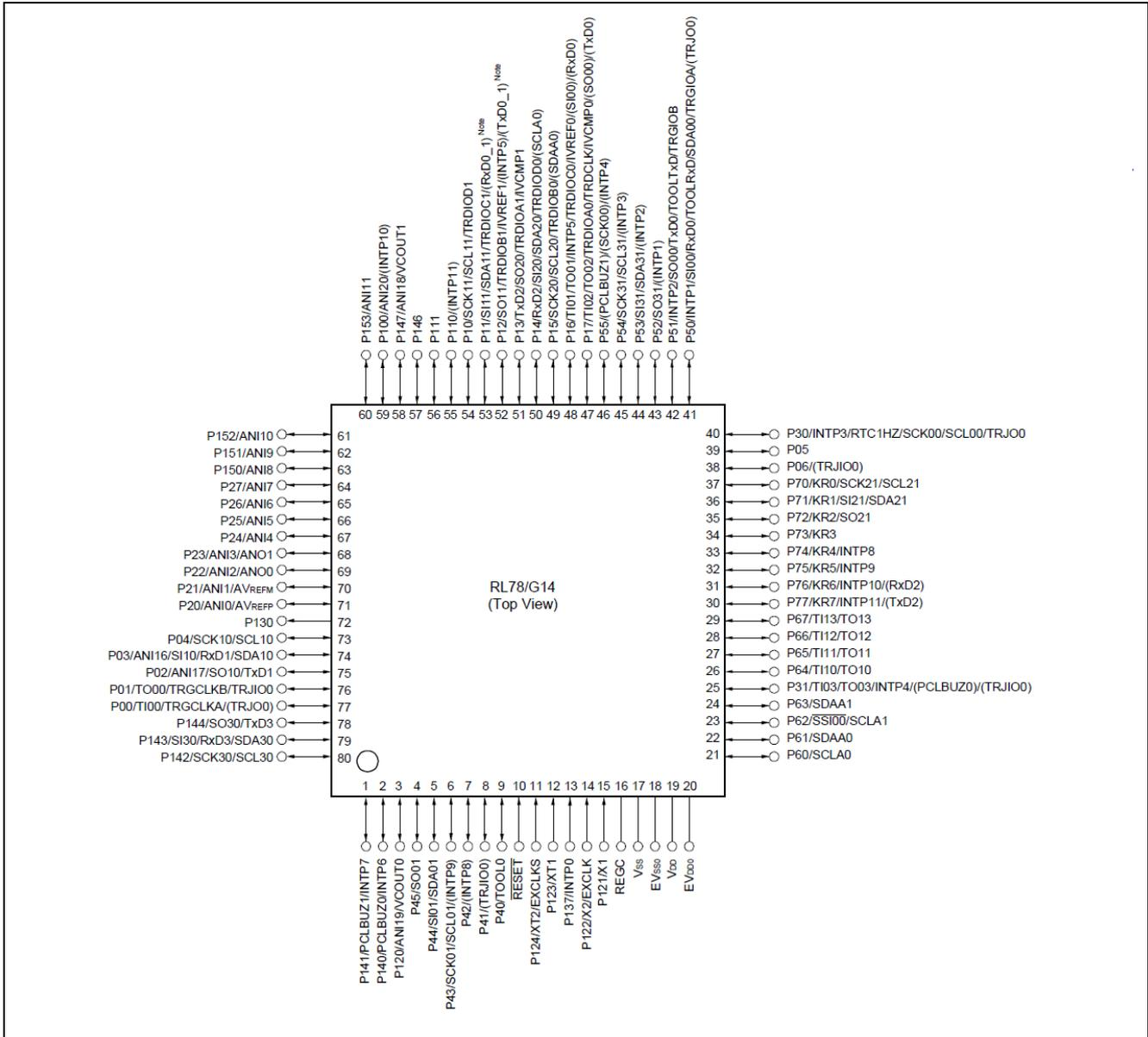
Figure 2.2 RL78/G14 (80-pin products) Pin Configuration
