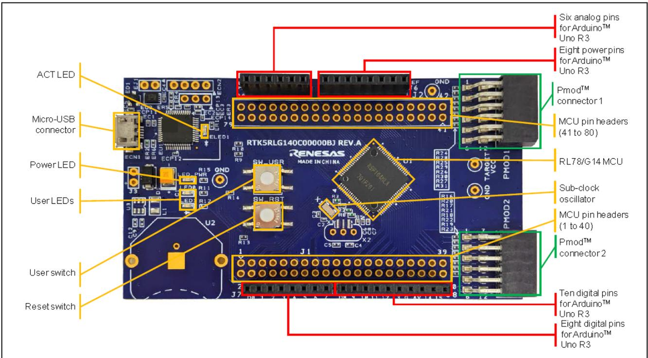
Figure 4.2 RL78/G14 FPB Board Layout (Top Side)
