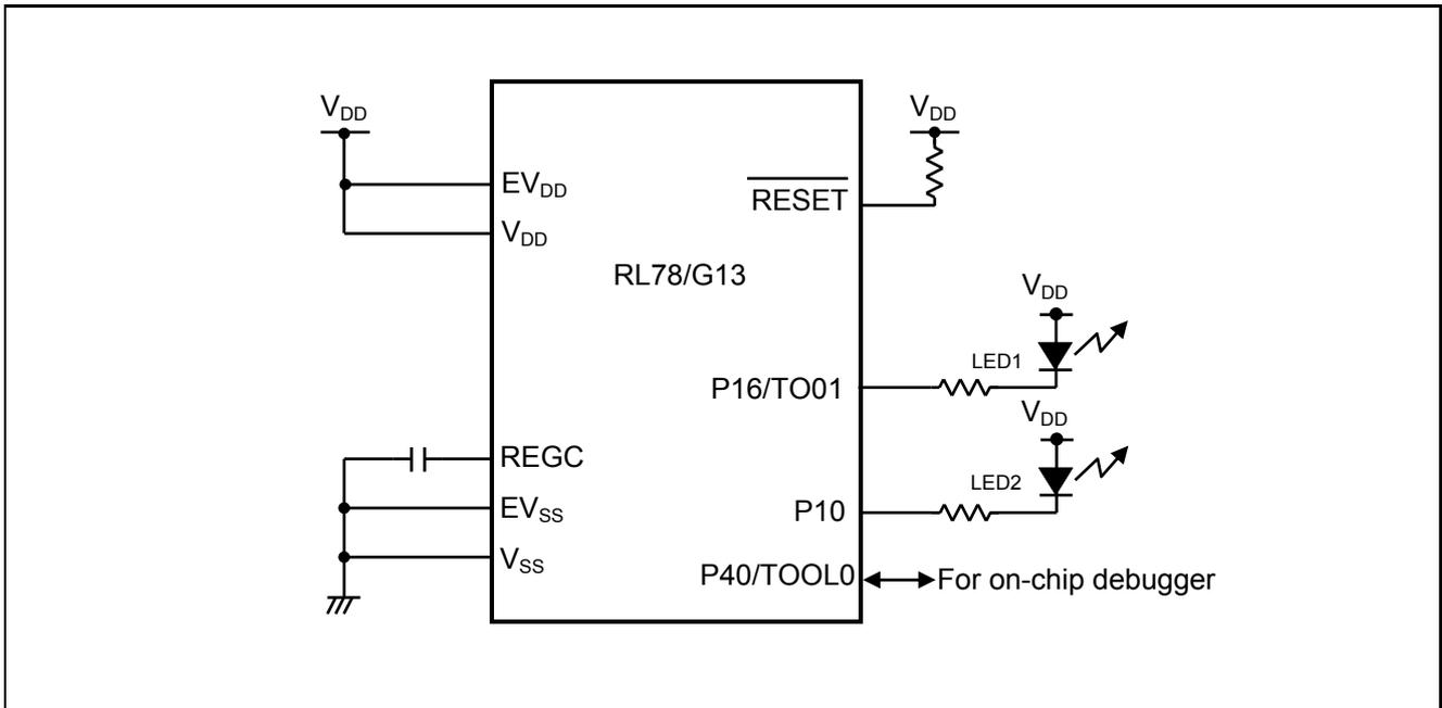
**Figure 4.1 Hardware Configuration**
