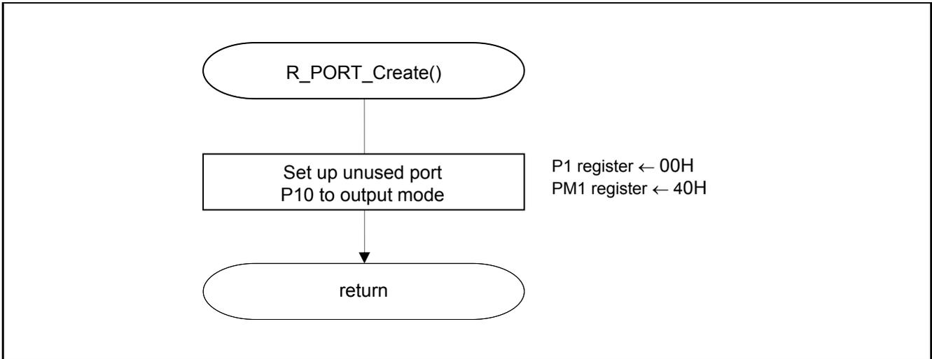
**Figure 5.4 I/O Port Setup**
