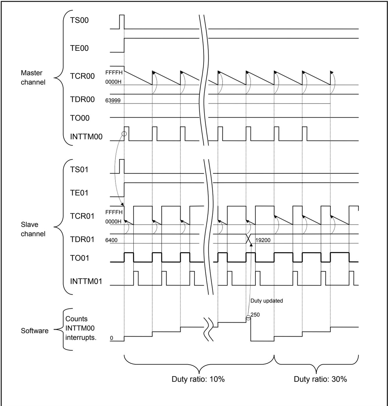
Figure 1.2 Simplified Timing Chart for PWM Output Operation
