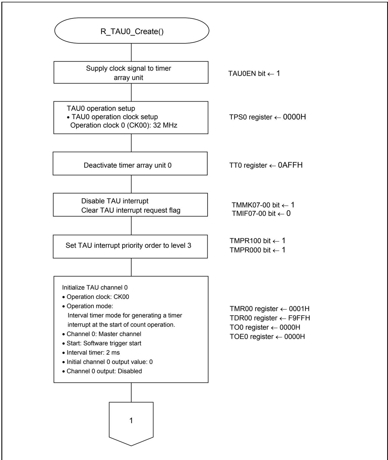
Figure 5.6 Timer Array Unit Setup (1/2)
