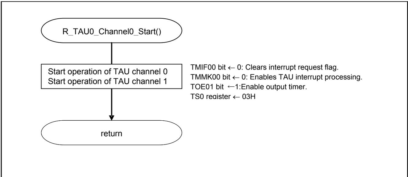
**Figure 5.10 Timer Array Unit Startup**
