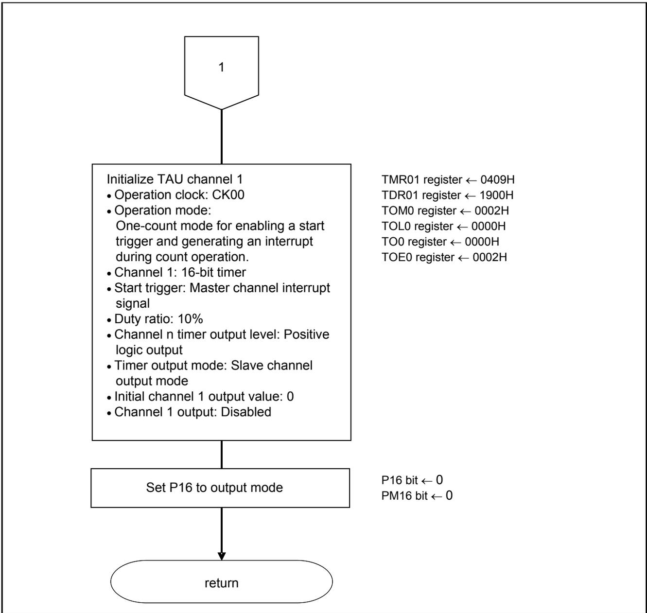
Figure 5.7 Timer Array Unit Setup (2/2)
