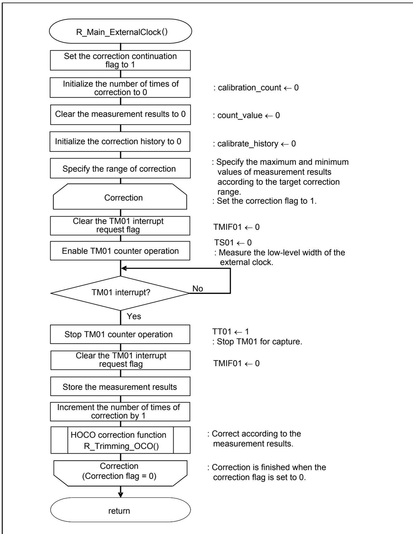
Figure 5.14 Calibration with External Input Clock
