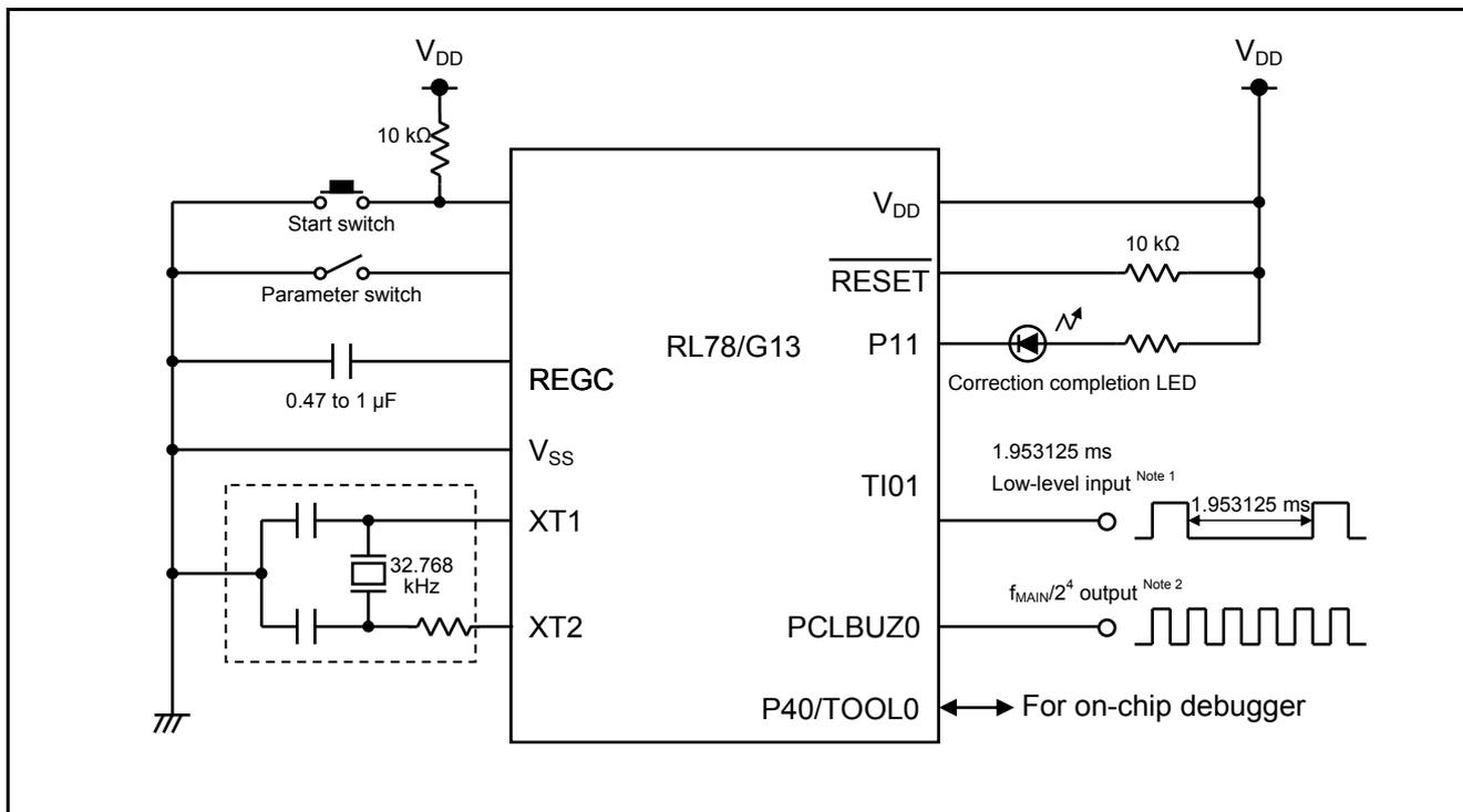
**Figure 4.1 Hardware Configuration**
