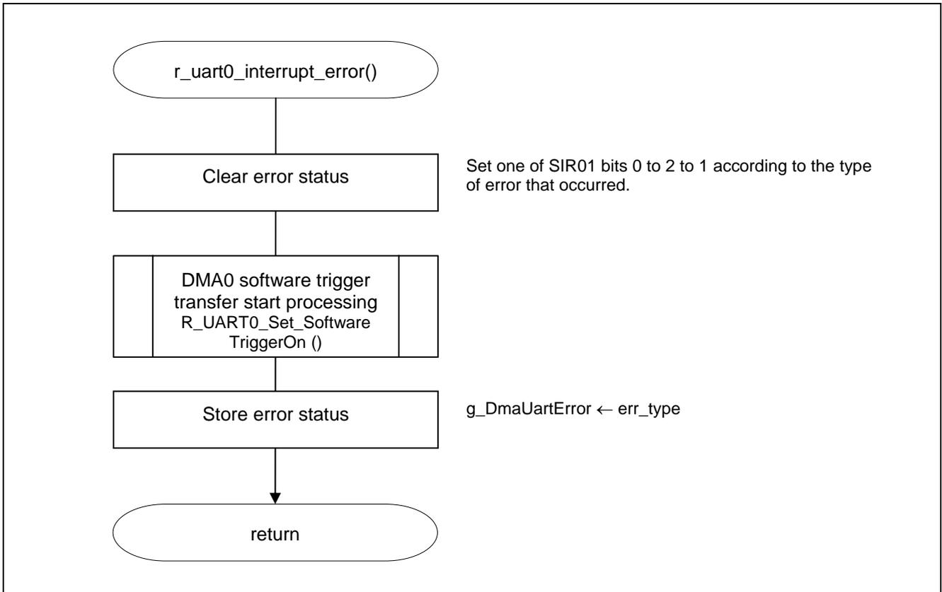
**Figure 5.13 UART0 Reception Error Interrupt Processing**
