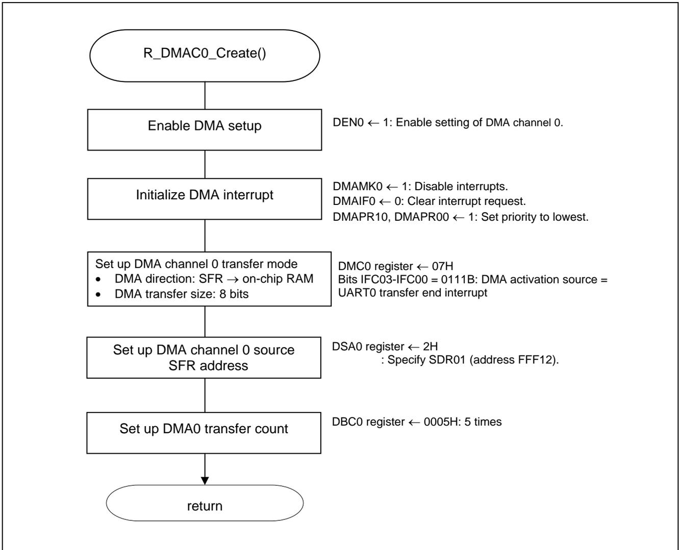
**Figure 5.8 DMA Controller Initialization**
