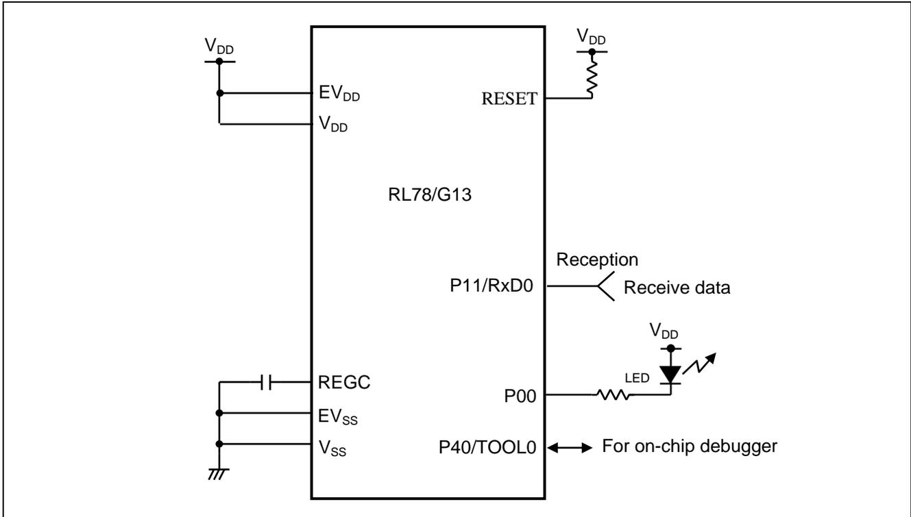
**Figure 4.1 Hardware Configuration**
