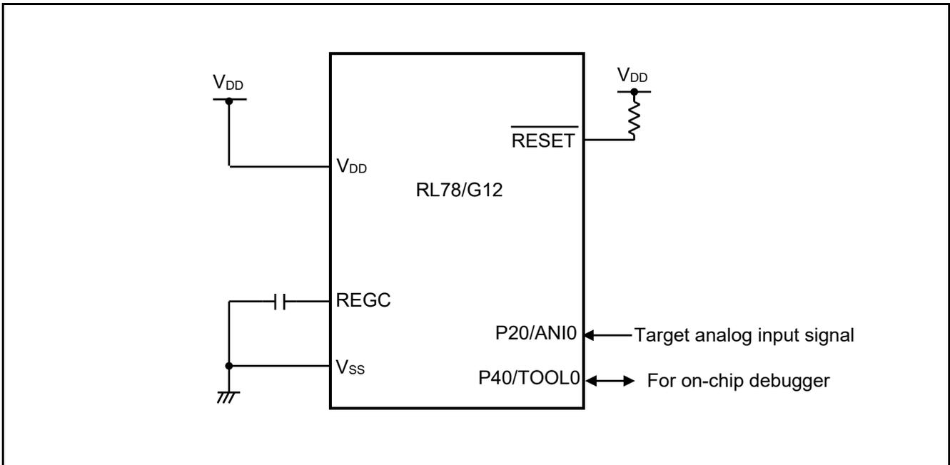
**Figure 4.1 Hardware Configuration**
