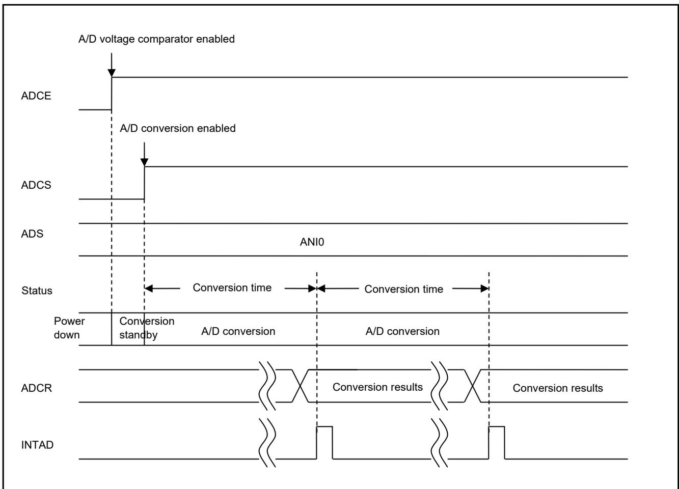
**Figure 1.1      Outline of the A/D Converter Conversion Processing**
