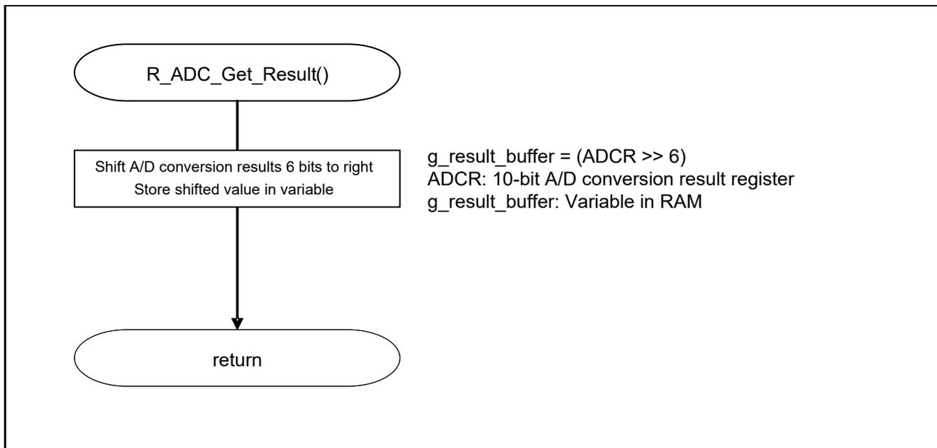
Figure 5.11 Storing the A/D Conversion Results in RAM
