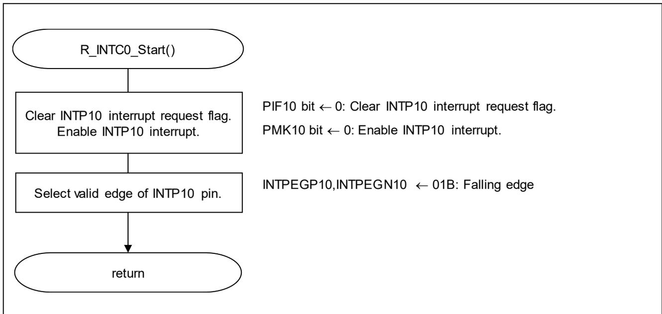
Figure 5.17 External Interrupt Operation Starting Function
