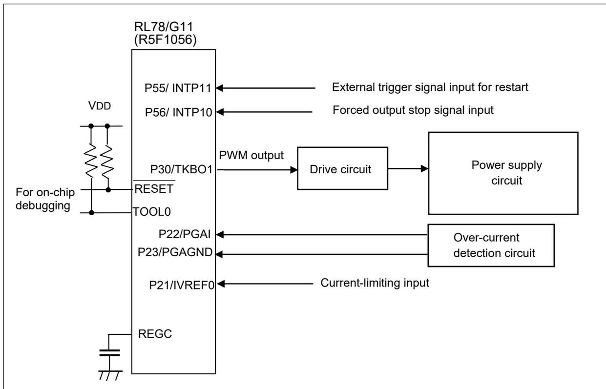
Figure 4.1 Hardware Configuration
