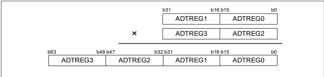
**Figure 1-6 Register Used in Multiply Mode (32 bits data)**
