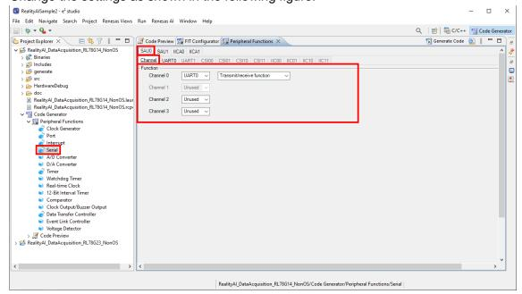
5. Select [Serial] tree and [SAU0] [UART0] [Receive] tab. Change the settings as shown in the following figure.
