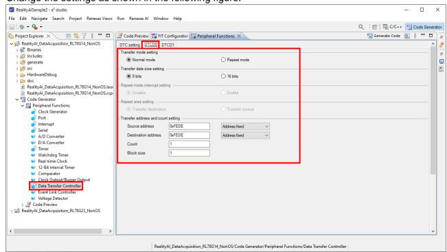
9. Select [Data Transfer Controller] tree and [DTC setting] tab. Change the settings as shown in the following figure.
