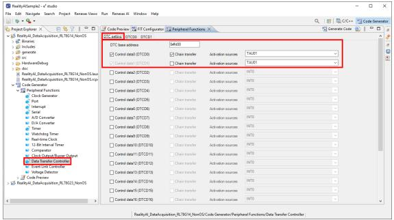
8. Select [Data Transfer Controller] tree and [DTC0] tab. Change the settings as shown in the following figure.
