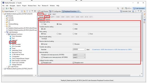
6. Select [Serial] tree and [SAU0] [UART0] [Transmit] tab. Change the settings as shown in the following figure.
