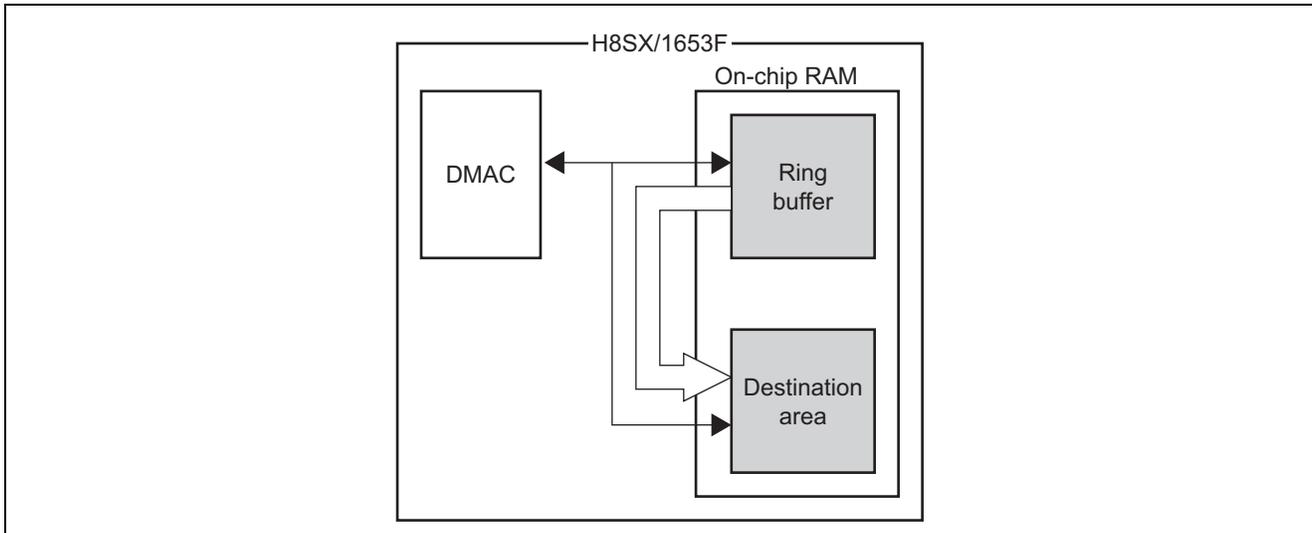
**Figure 1 Ring Buffer Processing by DMAC Extended Repeat Transfer**
