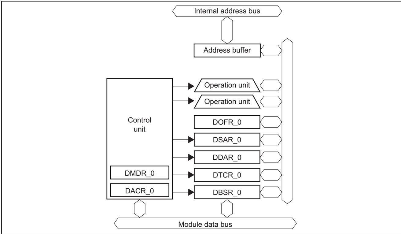
Figure 2 Block Diagram of DMAC
